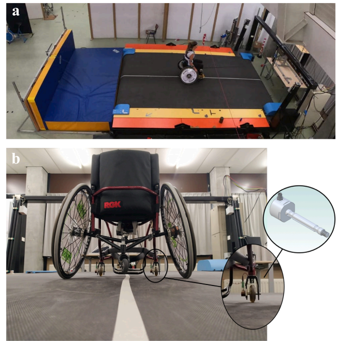
Fig. 1. a-b. Measurement set-up during the treadmill sessions. The custom-made load pins were integrated in each of the castor wheels (normal castor wheel axle were replaced by the load pins).
