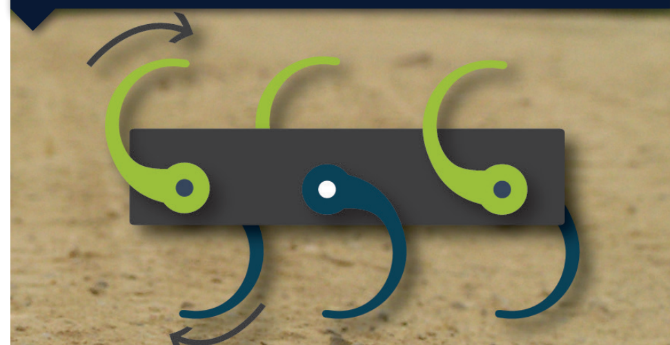
Figure 2e: Zebro uses an alternating tripod walking gait
