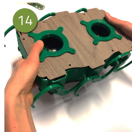
14. Click the top plate onto the robot
