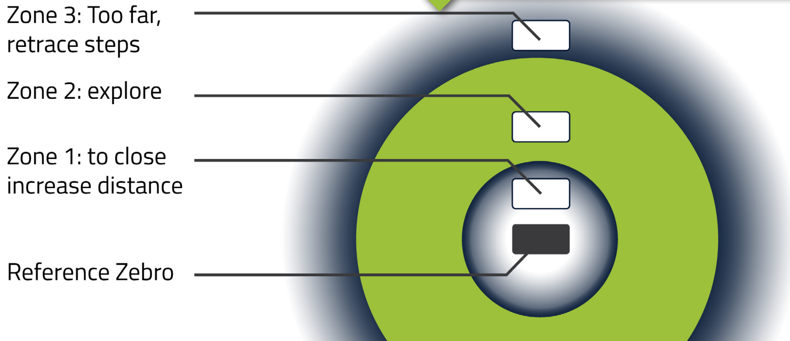
Figure 4e: Distance measurements in swarming
