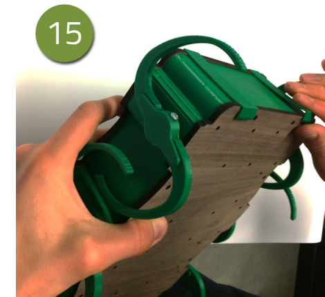
15. Click the clamps onto the sides - Finished!
