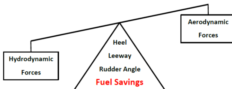
Figure 3: The force balance for the performance prediction program
