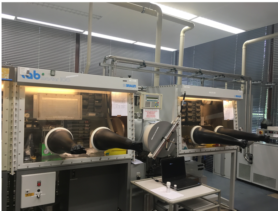
Figure 3.1: Glove box in which polymer electrolyte synthesis took place
