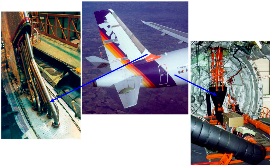
Figure 6. A320 HLFC Fin Flight Test of 1998.
