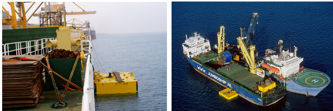
(a) Pontoon attached to the vessel in the harbour. (b) Lifting operation with a pontoon on calm sea.
