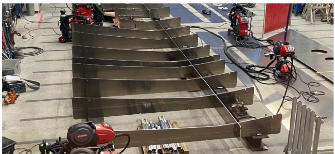
Figure 16: The templates aligned and welded to the H-beams.
