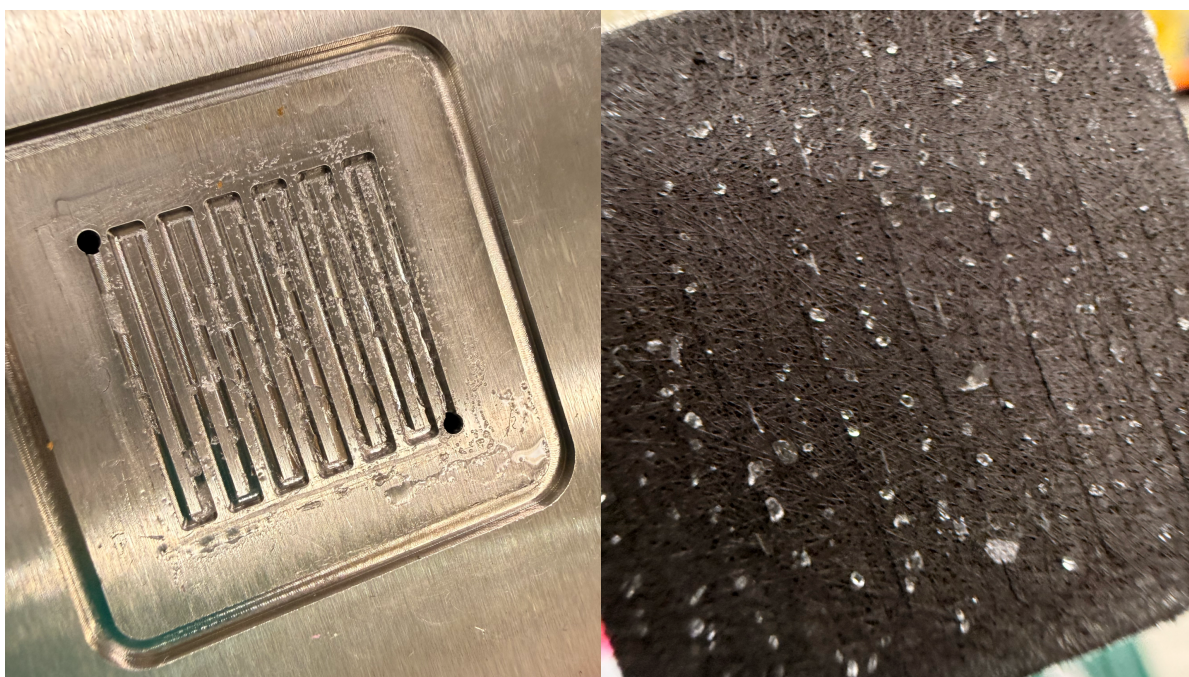
Figure B.1: Salt formation in flow field and on GDE cathode after running the Fumasep membrane chronopotentiometry tests.
