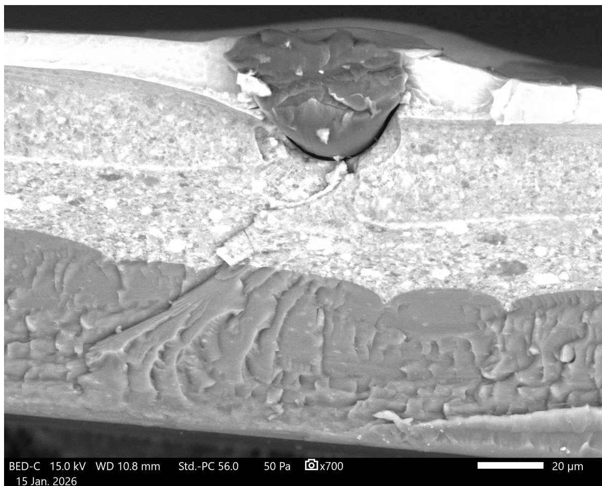
Figure B.5: SEM image of the tested Fumasep BPM. The picture shows an almost symmetrical BPM, with a thickness of about 100 \mu\text{m} .
