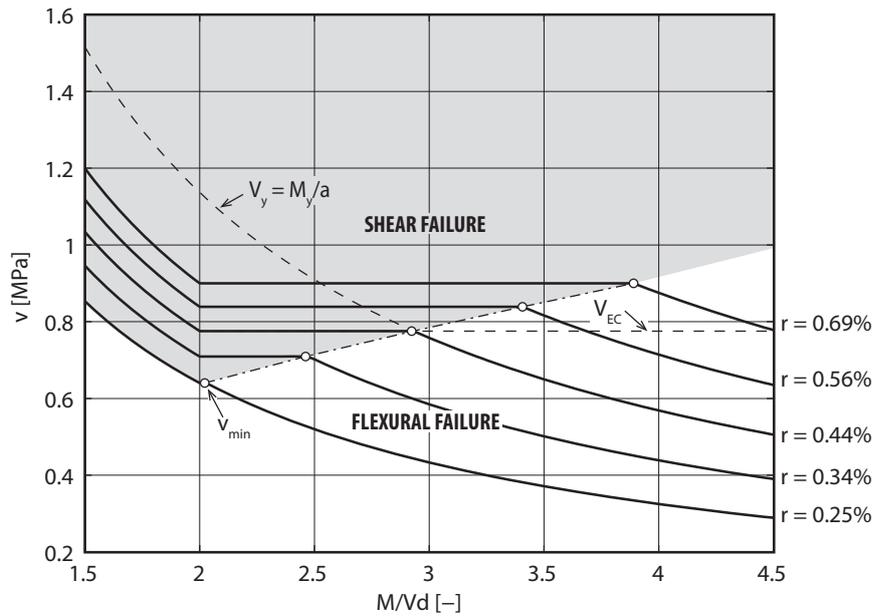
**Fig. 1.** Determination of  $v_{\min}$  according to Eurocode.
