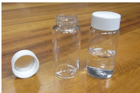
Figure 2.3. Liquid scintillation vials (LSVs) with Al-lined cap. A sample with 10 mL TBA liquid is shown on the right.
