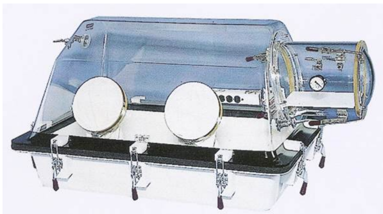
Figure 2.2. The glove box PlasLabs GB818 used for deaerating TBA liquid.
