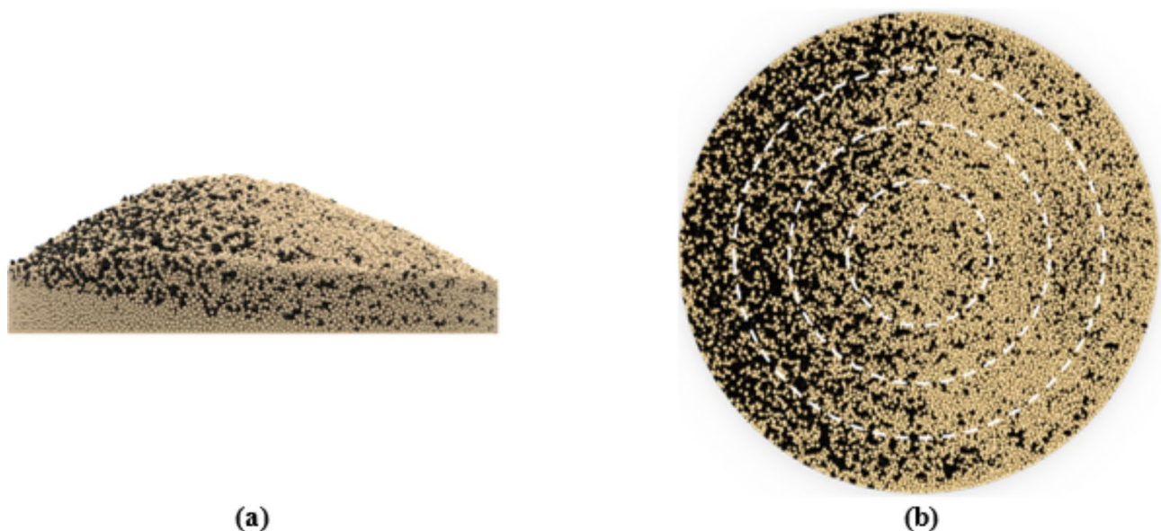
Fig. 3. (a) Side view of the heap formed within the receiving bin, (b) radial bins used to quantify radial segregation.
