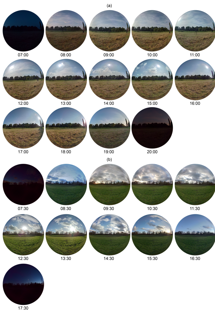
Figure 4.6: sRGB representations of illumination maps measured at a 60-minute interval via a Panono spherical camera.
