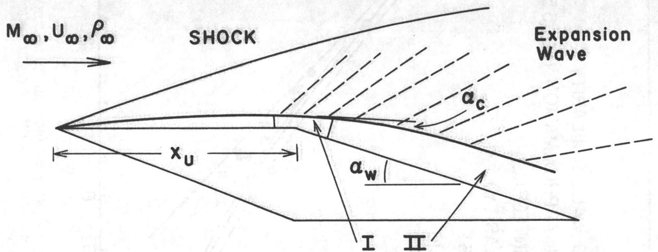
FIGURE 1: PROPOSED MODEL FOR HYPERSONIC FLOW AND SMALL TURNING ANGLES  $\alpha_w$ . REGION I IS THE AREA WHERE THE BOUNDARY LAYER EQUATIONS ARE PRESUMED TO BE INAPPLICABLE, AND REGION II IS THE DOWN-STREAM INTERACTION REGION.
