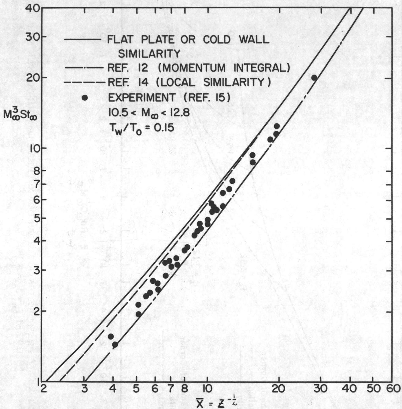
FIGURE 3: COMPARISON OF VARIOUS APPROXIMATE THEORIES FOR HEAT TRANSFER TO A FLAT PLATE IN HYPERSONIC FLOW WITH EXPERIMENT.
