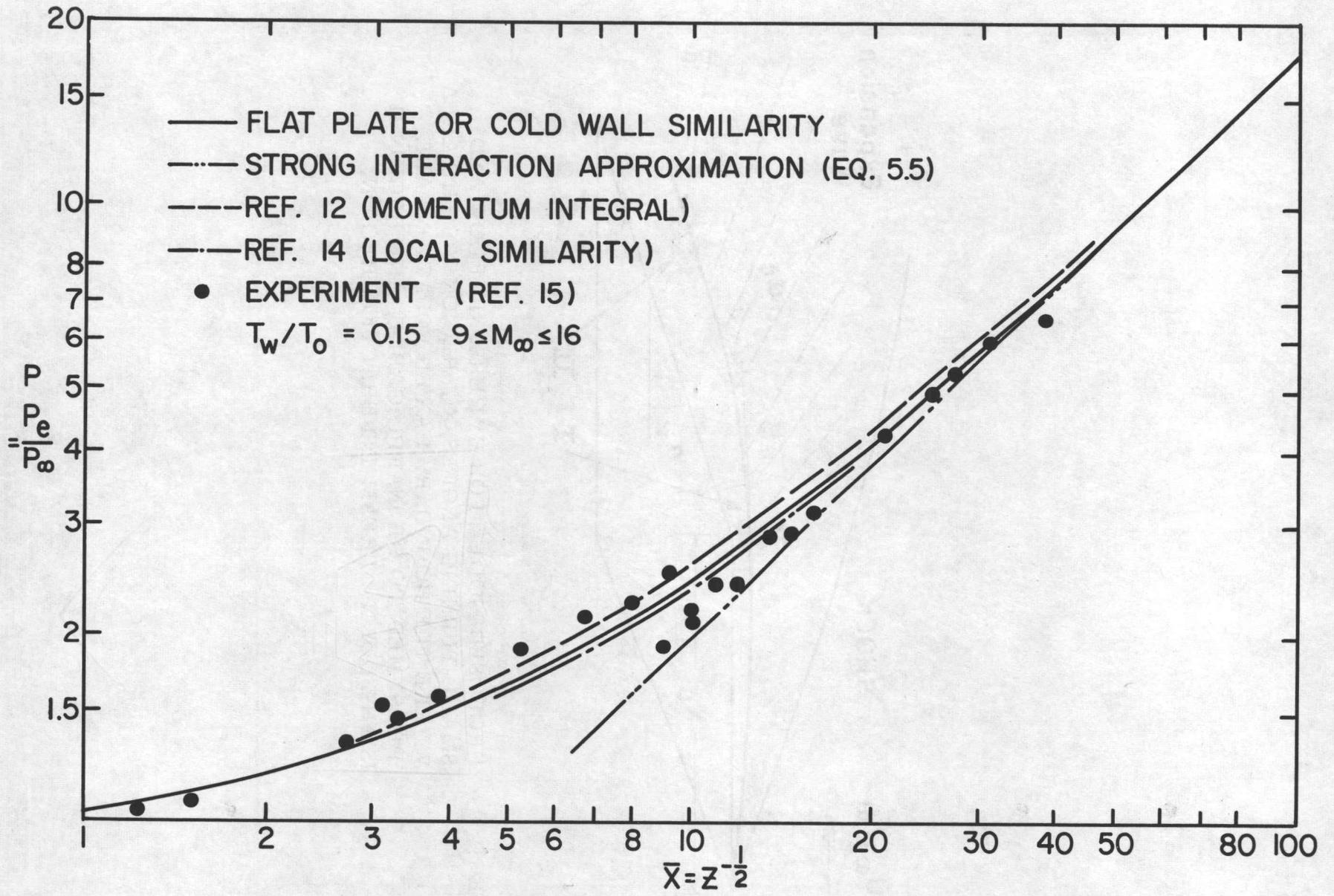
FIGURE 2: COMPARISON OF VARIOUS APPROXIMATE METHODS FOR PREDICTING THE PRESSURE DISTRIBUTION ON A HYPERSONIC FLOW WITH EXPERIMENTAL RESULTS.
