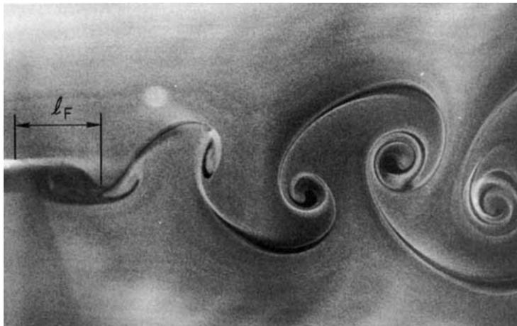
**Figure 2.2:** Vortex Shedding behind a cylinder showing  $l_F$ , taken from [15]
