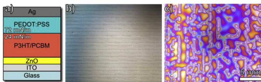
Fig. 1. A schematic representation of the inverted OPV stack (a), A picture of an inkjet printed layer of our standard CH8000 based, inkjet printing formulation (b) and a printed layer of CH8000 + 0.1 wt% Capstone FS-3100 (c). Both printed layers show inhomogeneous layers due to dewetting of the ink in the substrate.
