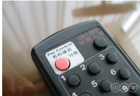
Figure 4: In this hotel remote control the pay-per-view button has the appearance (red) and position (upper left) that is usually reserved for the on-off button, thus prioritizing sales over adhering to user interface conventions.
