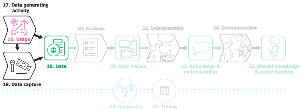
Figure 60: The generation of data about usability issues (19) requires an activity through which the data is generated (17) in which product usage occurs or is simulated (16), which is then captured (18).
