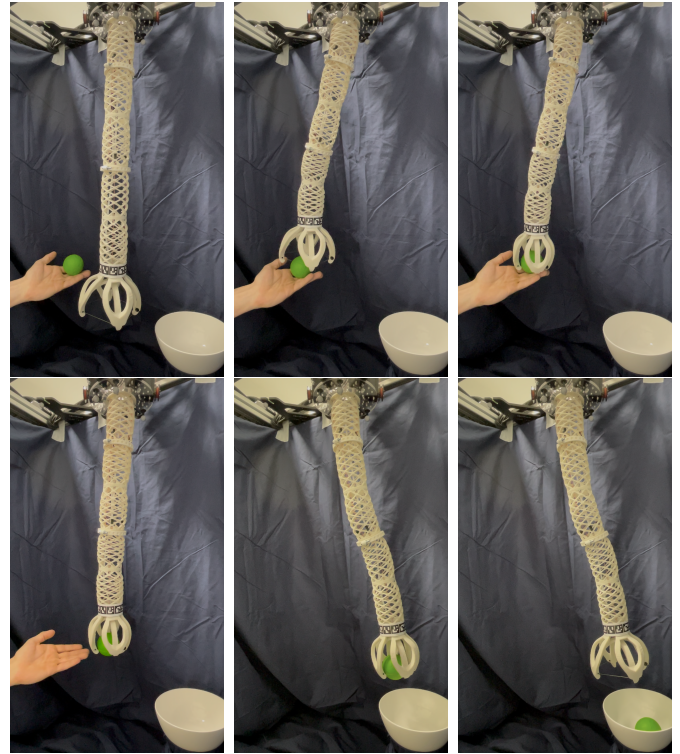
Fig. 13. The evolution of one of the performed use case tasks. The first image shows the starting position, the second and third show the handover task. The fourth and fifth image show the movement of the arm (with ball) towards to desired location. The last image shows the system when the task is just finished.
