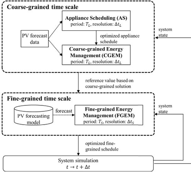
Fig. 6. Multi-time scale optimization flow of proposed framework.
