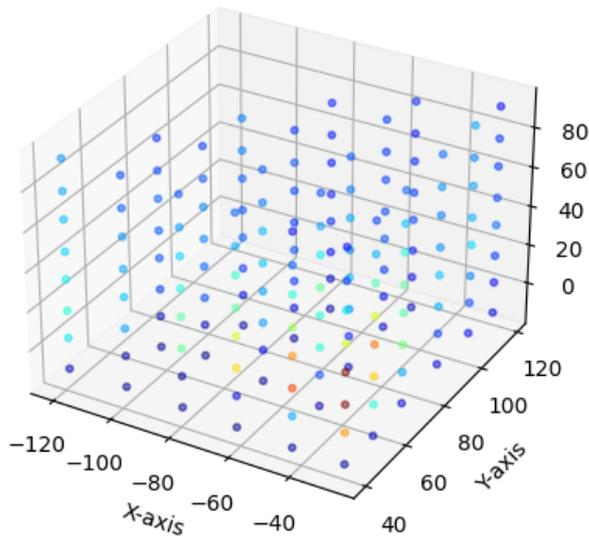
Figure 25: Measurement points; AP orientation, Acquisition mode, Without lead screen. The colour of the dots are dependent on the Doserate value, where dark blue is low and dark red is high.
