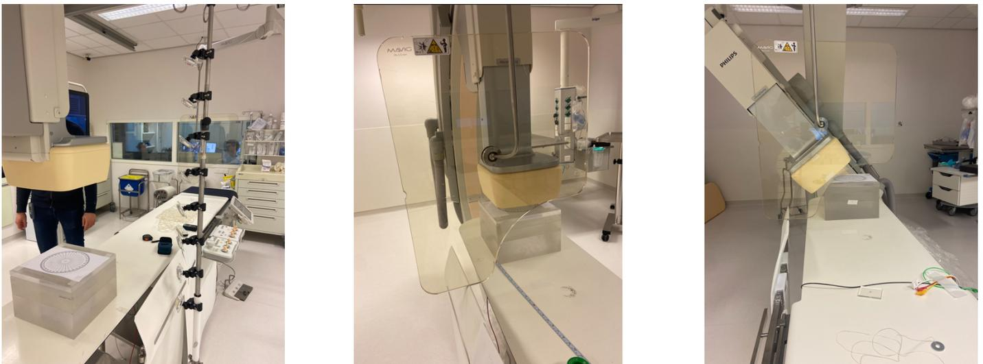
Figure 15: Illustration of the setup. Left: Pole and badges oriented towards the center of the phantom. Middle: The setup with the C-arm in AP view and with the lead screen. Right: The setup with the C-arm in a 40° tilted view and with the lead screen.
