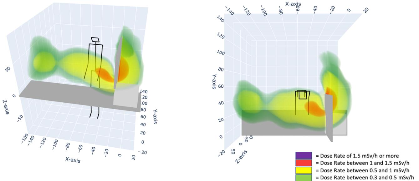
Figure 12: Measurement data without the shield combined with the estimated attenuation of the lead screen. AP orientation C-arm, Acquisition mode. Lead screen placed 0 cm from the phantom.
