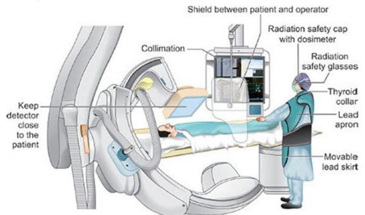
Figure 1: Catheterisation Laboratory with possible protective measure
