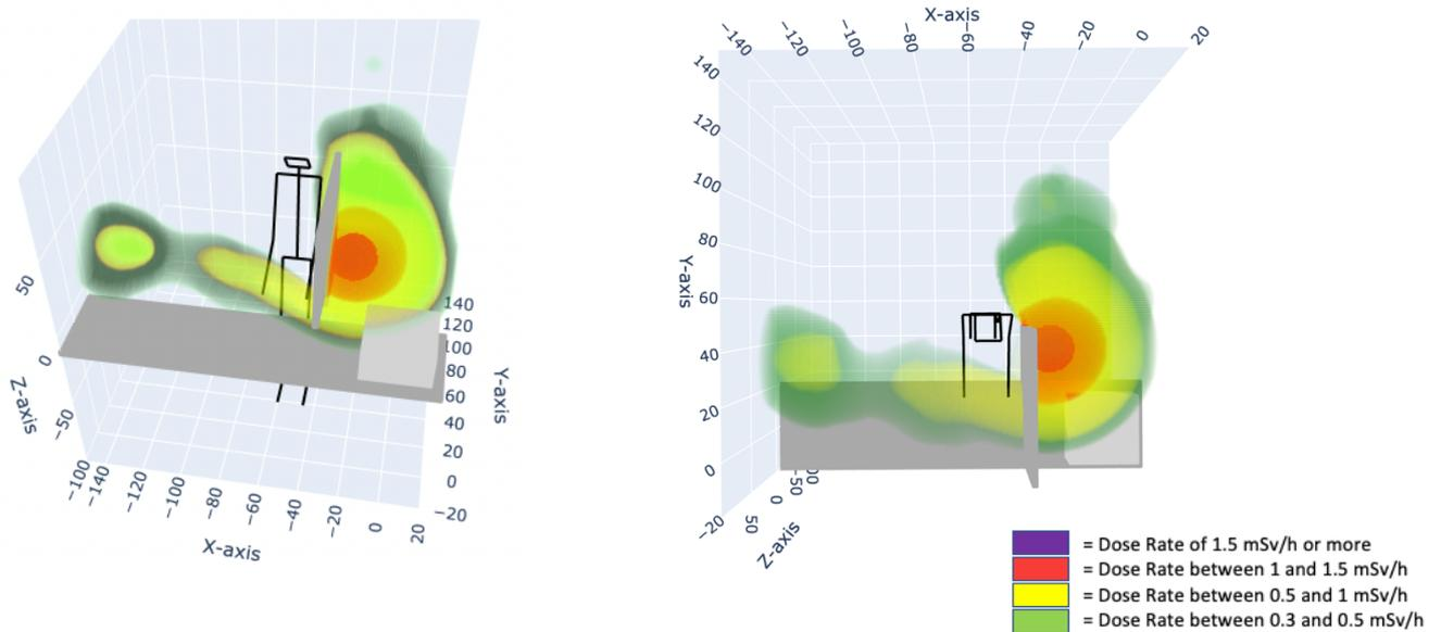
Figure 11: Measurement data without the shield combined with the estimated attenuation of the lead screen. AP orientation C-arm, Acquisition mode. Lead screen placed 20 cm from the phantom.
