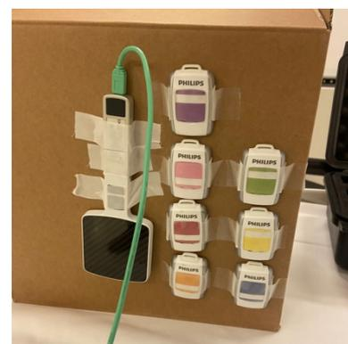
Figure 3: Measurement set-up for preliminary tests. On the left is the RaySafe X2 dosimeter. On the right are the Philips DoseAware Dosimeters
