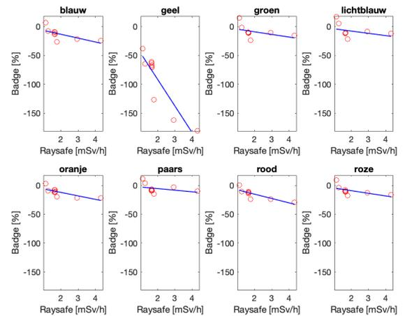
Figure 4: Percental difference between the dose rate measured by the Raysafe and by the DoseAware badges
