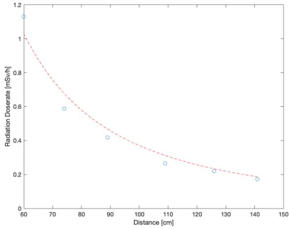
Figure 22: AP orientation C-arm, Acquisition mode, With lead screen (measurements 105 cm above the ground)
