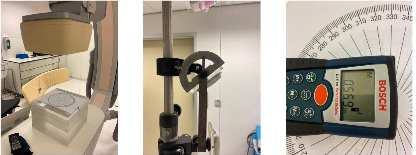
Figure 16: Establishing the correct setup. Left: Alignment of the C-arm with the phantom. Centre: Adjustment of the badge's angle using a weighted string and a protractor. Right: Determination of the pole's orientation and distance in relation to the phantom.
