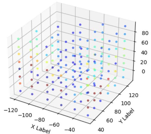
Figure 30: Measurement points; 40° tilted orientation, Acquisition mode, With lead screen. The colour of the dots are dependent on the Doserate value, where dark blue is low and dark red is high.
