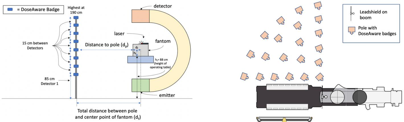
Figure 7: Measurement set-up. In the left figure the lateral view is showed with the 8 badges on the pole, the phantom and the C-arm. The right figure shows the locations of the pole in the room, where the pole for every measurement is directed at the phantom.
