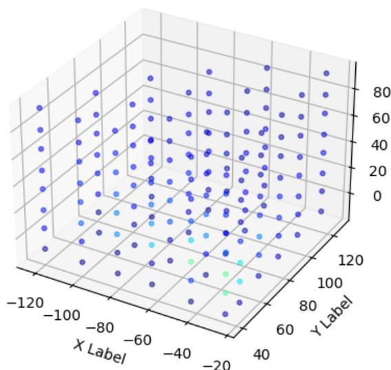
Figure 32: Measurement points; 40° tilted orientation, Fluoroscopy mode, Without lead screen. The colour of the dots are dependent on the Doserate value, where dark blue is low and dark red is high.
