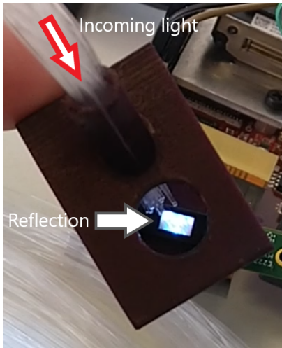
Figure 7: DMD reflecting light coming from optic fibers
