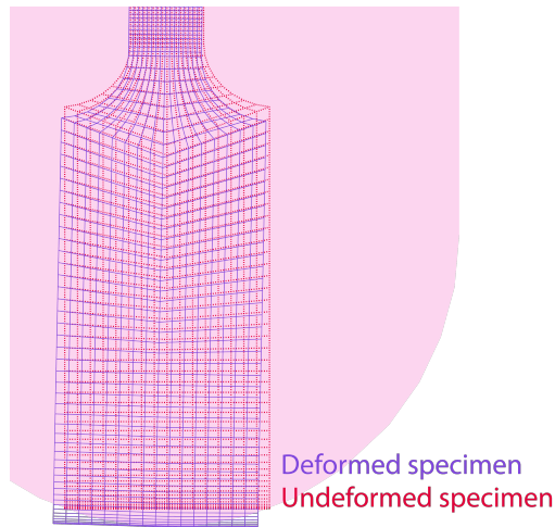
Figure 4.17: The specimen slips away from under the deformable drophead
