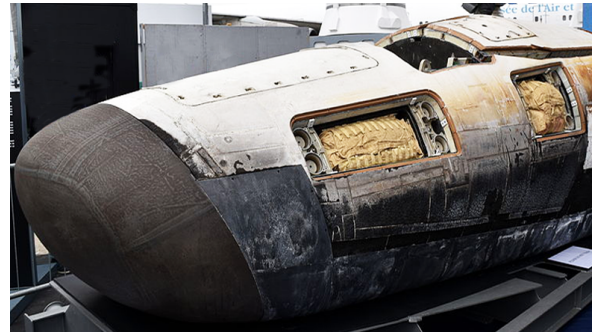
Figure 1.2: Photo of the IXV after reentry. Evident paint job and TPS damage is shown b .
