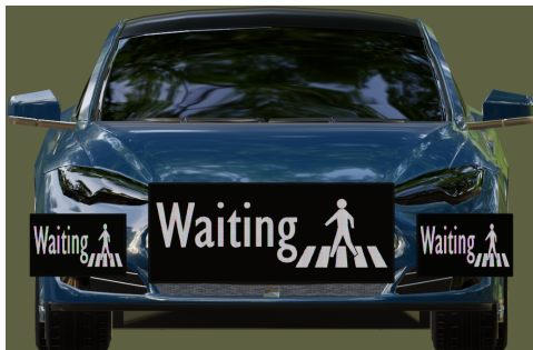
(a) Front view showing the positioning of the eHMI panels on the car model.
