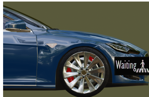
(b) Side view showing the positioning of the eHMI panels on the car model.
