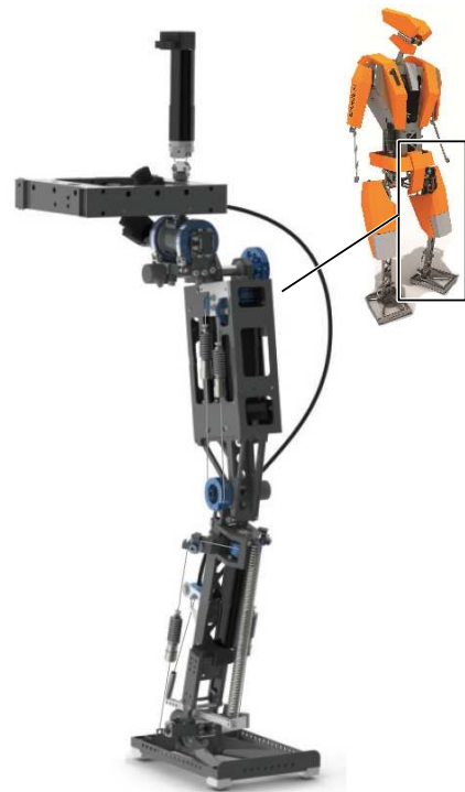
Fig. 1. A CAD model of the TULip humanoid robot, showing the construction of the six degree of freedom leg.
