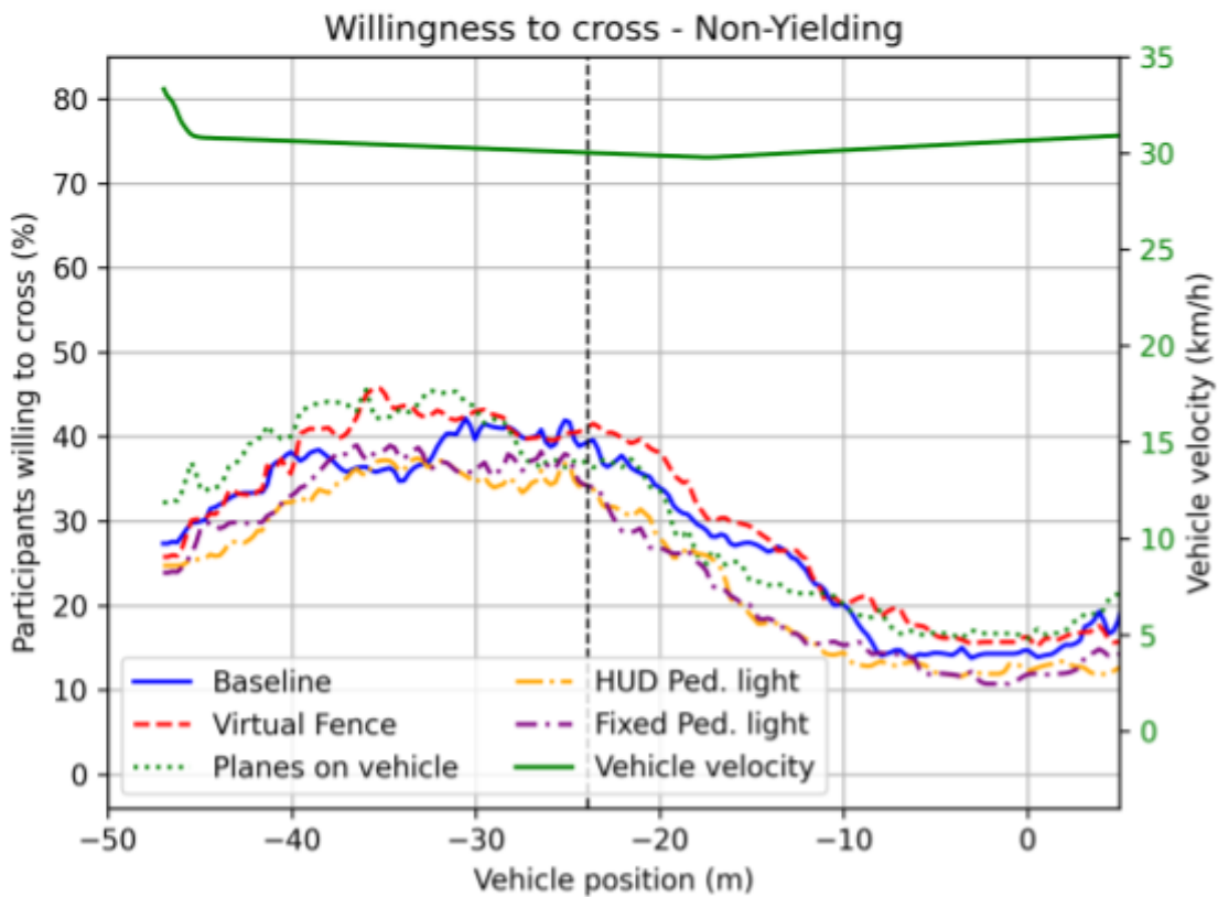
Figure 9: Willingness to cross - The percentage of participants indicating with the button that they are willing to cross during vehicle approach. The vertical lines represent the triggers at which the interface activated (black dotted), the vehicle decelerated (red dotted) and the vehicle stopped (green dotted).
