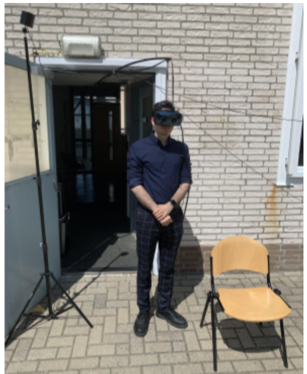
Figure 7: Participant wearing the tethered Varjo XR-3 HMD. One SteamVR base station can be seen on a tripod in the left of the image.
