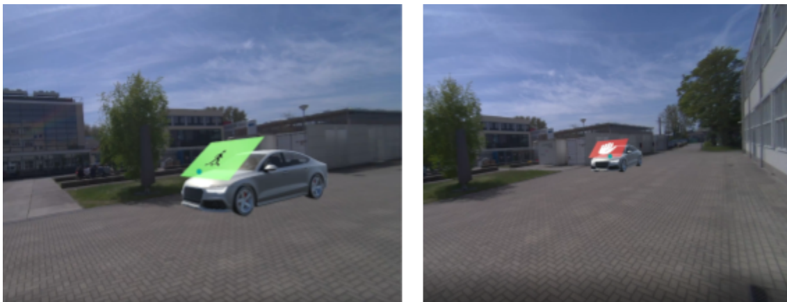
Figure 4: Planes on vehicle interface augmented at experiment location from right eye view. Left: yielding (green) state; Right: non-yielding (red) state.
