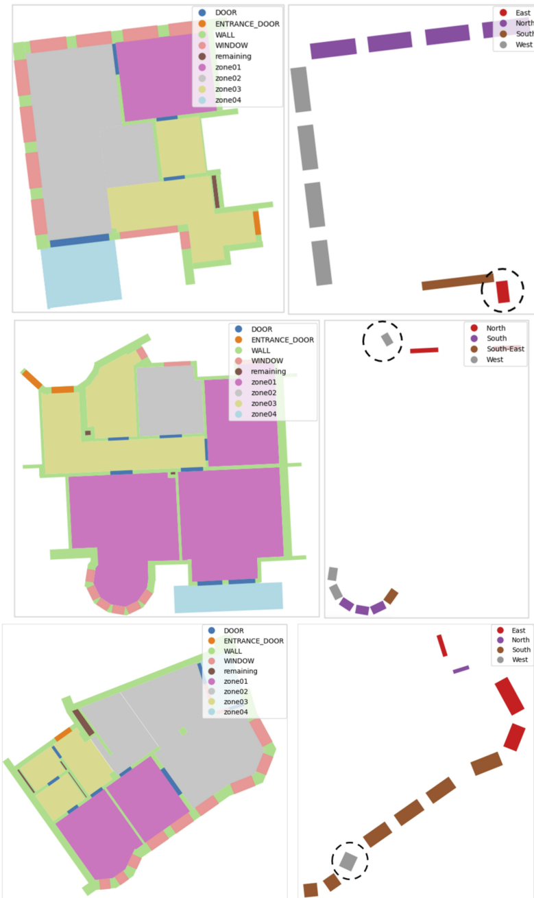
Figure 8. Examples of floor layouts in O-ESD with an incorrectly labeled window orientation in the window orientation maps
