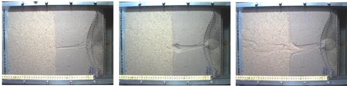
Figure 2.16. Pipe formation in laterally heterogeneous sands (fine downstream, coarse upstream)
