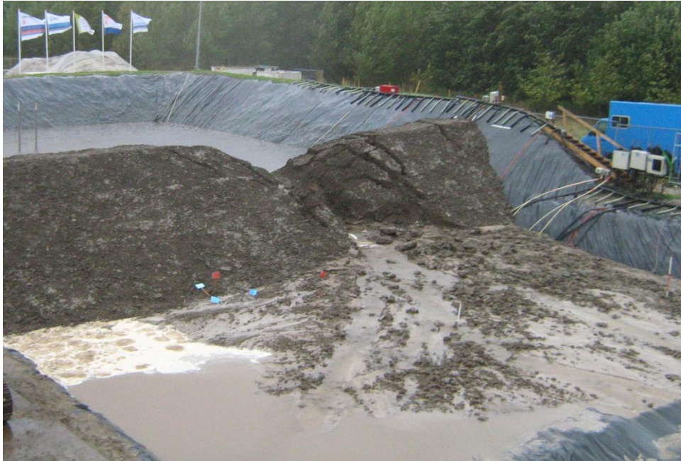
Figure 3.4. Failed dike in full-scale experiment (scenario 1)
