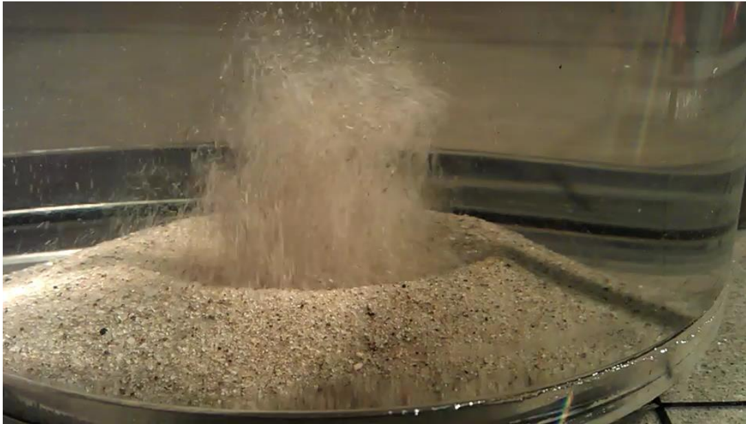
Figure 4.6. Example of sand crater and sand in transport
