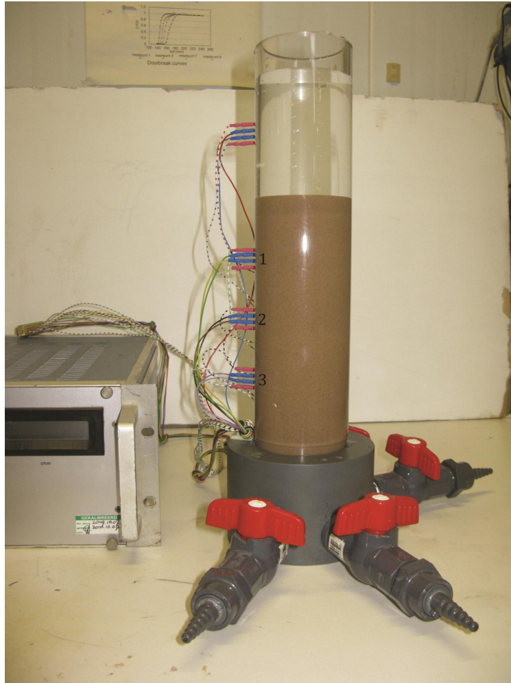
Figure 4.14. Column experiment to investigate the relationship between porosity and electrical resistance. The figure shows the locations of the copper needles.
