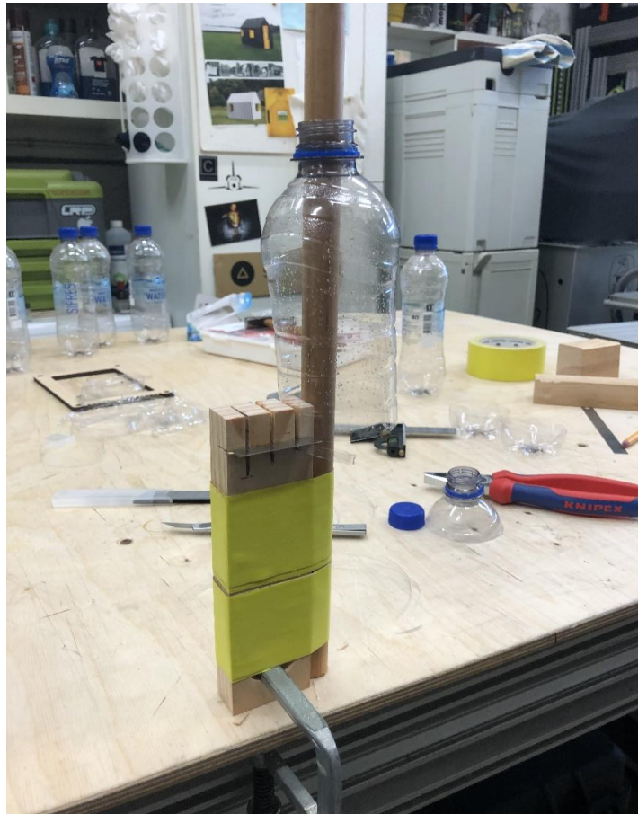
PET SLICER WITH 5MM, 10MM, 15MM SPACES. G-CLAMP ATTACHED, STICK TO GUIDE THE SLICER
