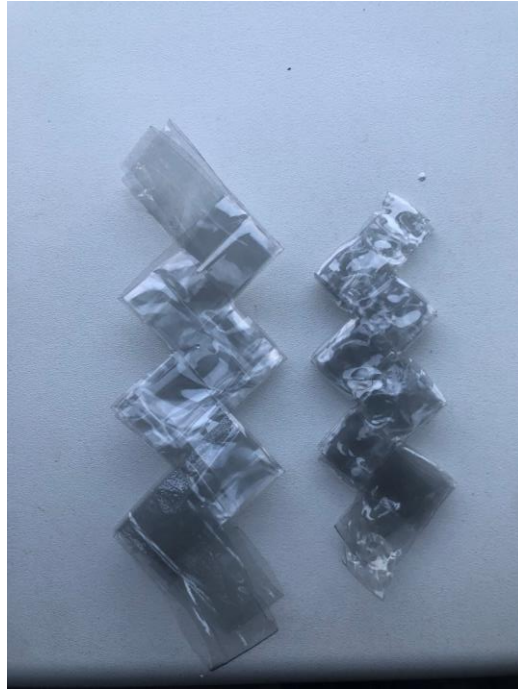
VISUAL COMPARISON BETWEEN PET WITHOUT HEAT AND WITH IRON HEAT
