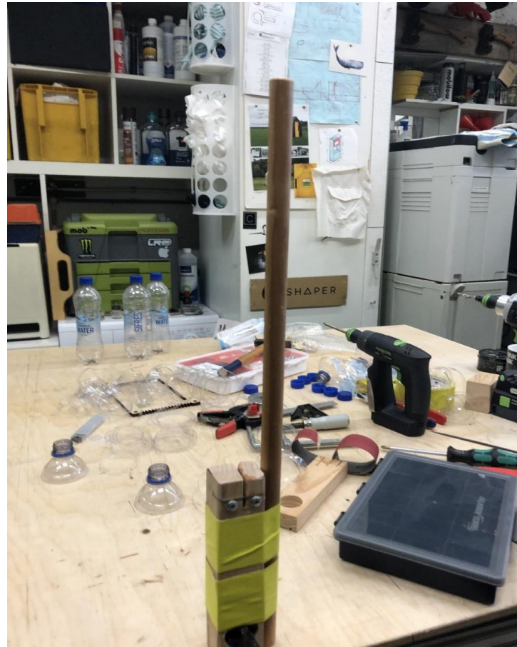
PET SLICER FOR 10MM THREAD
