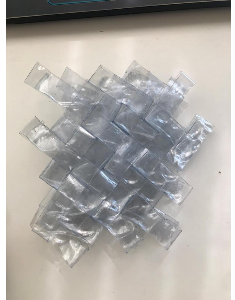
MULTIPLE WOVEN LAYER WITH IRON HEAT APPLIED
