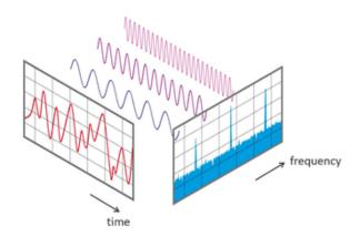
Figure 3.2: View of a signal in the time and frequency domain. Figure from Chac & Wriggers (2002).
