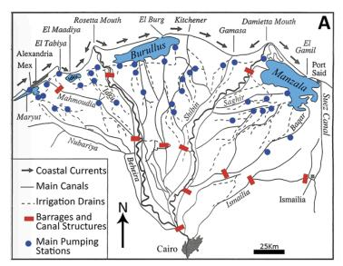
Figure A.7: Map of geographic features and network of major canals, drains, and pumping stations in the Nile delta. Figure from Stanley & Clemente (2017).
