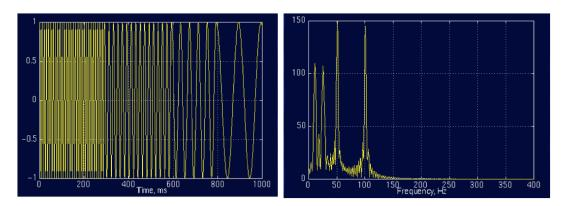
Figure 3.3: Time series and it's Fourier transform. Figure from Polikar (1996).
