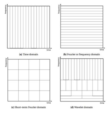
Figure 3.4: Schematic representation of the four different analyses of a signal. Figure from de Rooij (2017).
