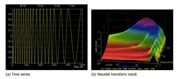
Figure 3.5: Time series and wavelet transform of the time series. Figure from Polikar (1996).
