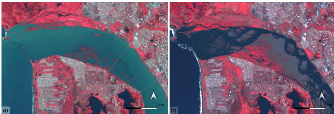
Figure II - 4: False colour satellite images of the mouth of the Biobío River. Dense vegetation (high infrared light reflection) is depicted in bright red. Images from LANDSAT 8 captured a) on the 31/08/2015 and b) on the 11/05/2015.
