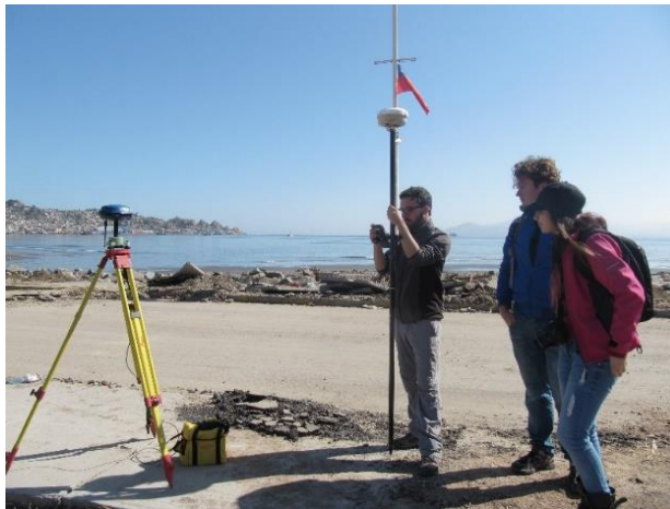
Figure III - 8: Fixed GPS on a tripod and a free GPS on a pole.
