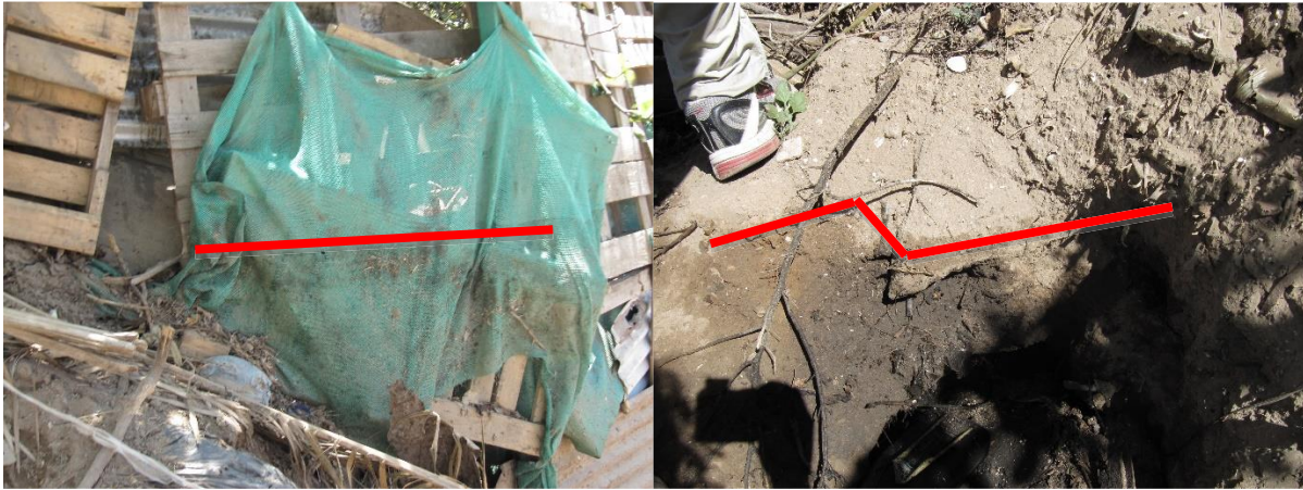
Figure III - 9: Left; waterline (marked red) on object. Right; end of run-up on a slope (marked red).
