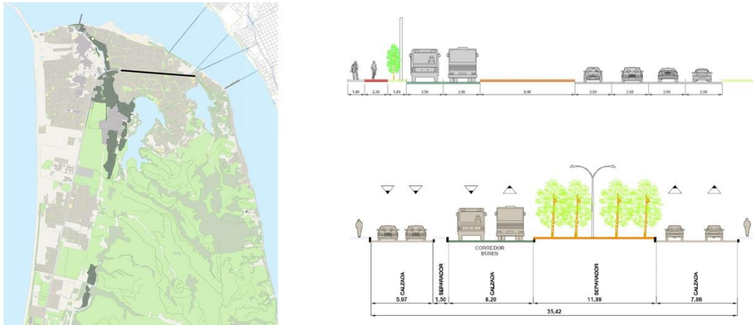
Figure I - 11: LRTB: Location of Pedro Aguirre Cerda, Existing road profile 3 , Improved road profile design 3
