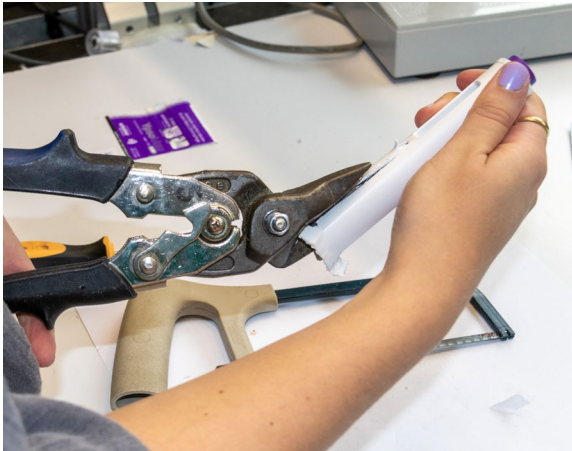
Fig. 85: I had to cut open the housing to separate it from the cover sleeve and the syringe holder.
