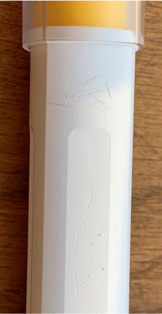
Fig. 60: I scratched the polycarbonate housing on purpose with a sharp stainless steel part. These scratches do not occur during normal use.
