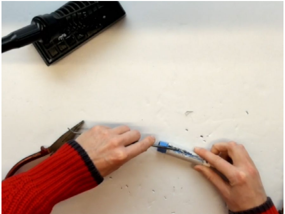
Fig. 90: To remove the housing, I broke it open by melting the plastic with a soldering iron.
