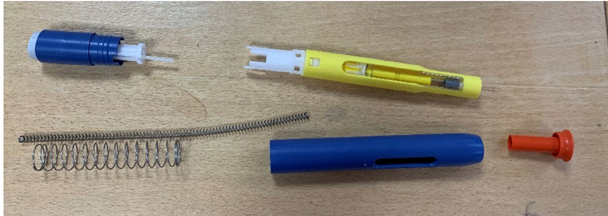
Fig. 89: After opening the housing, the Novartis autoinjector fell apart into subassemblies. This sped up the disassembly process.
