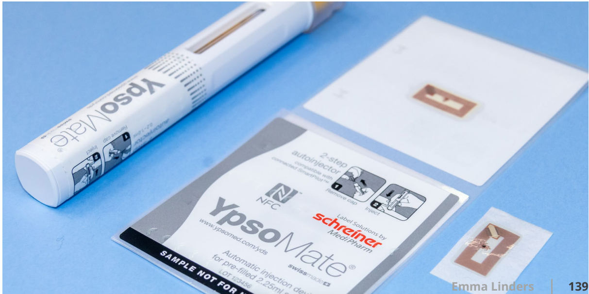
Fig. 105: A label with a laminated NFC tag inside it is glued around the housing of the YpsoMate.
