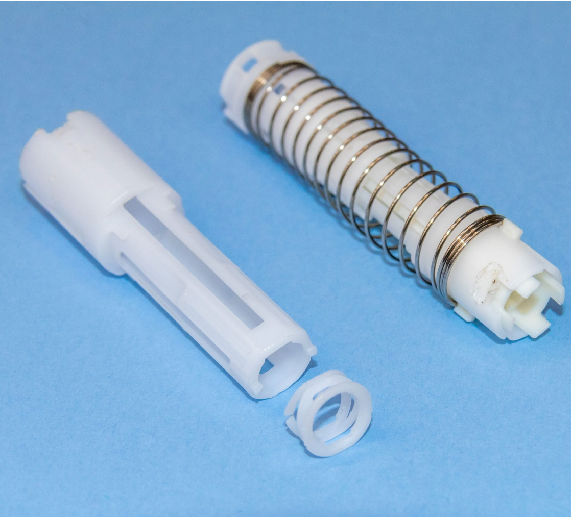
Fig. 59: The plastic spring broke of the Click Sleeve during manual disassembly.
