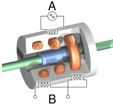
**Fig. 2.2.5 Cross-section of LVDT**
