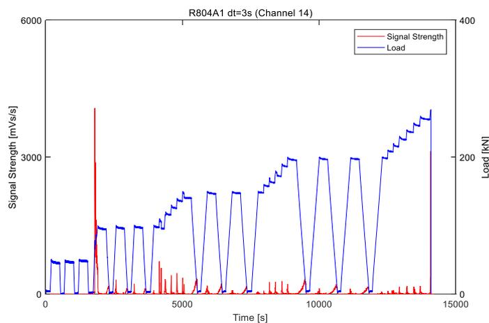
**Fig. 4.3.2 Load-time and SS-time curve of R804A1 (Channel 14  $dt=3s$ )**
