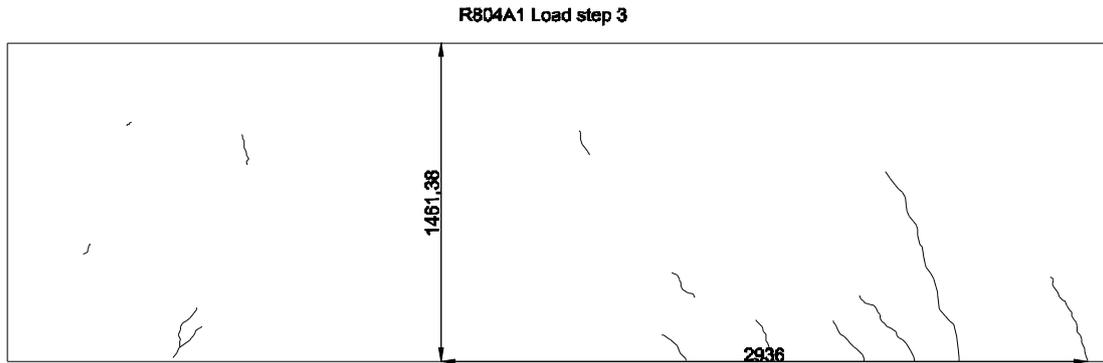
Fig. 5.2.12 Crack pattern of R804A1 load step 3
