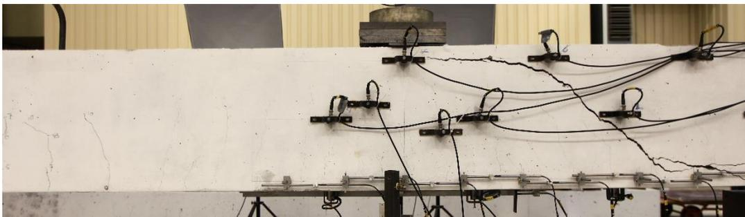
**Fig.A2. 3 Crack pattern of R501B1**
