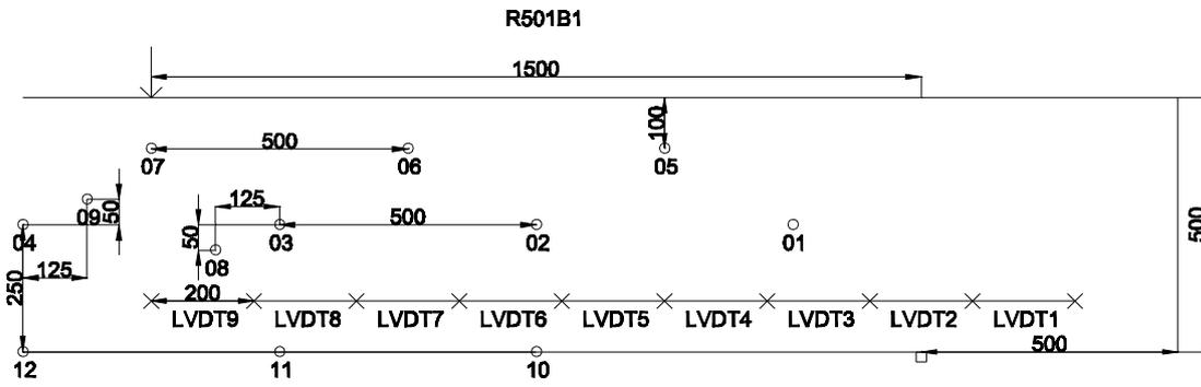
Fig.A2. 1 LVDT and AE grid (R501B1)
