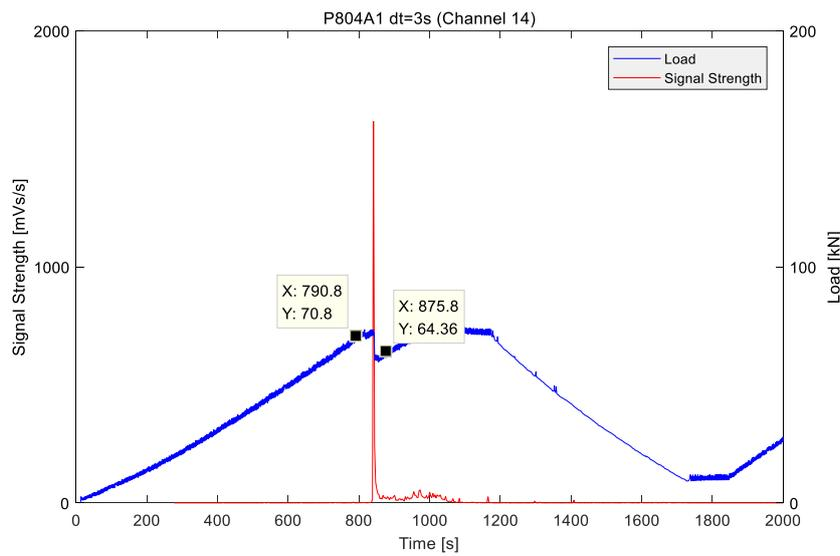
Fig.A2. 11 SS-time curve of P804A1
