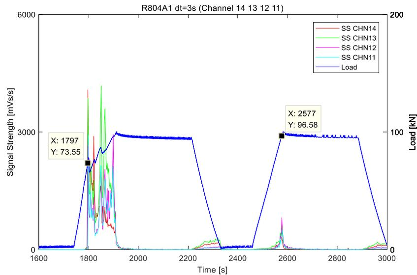
Fig. 5.2.1 Load and Signal strength against Time (R804A1)
