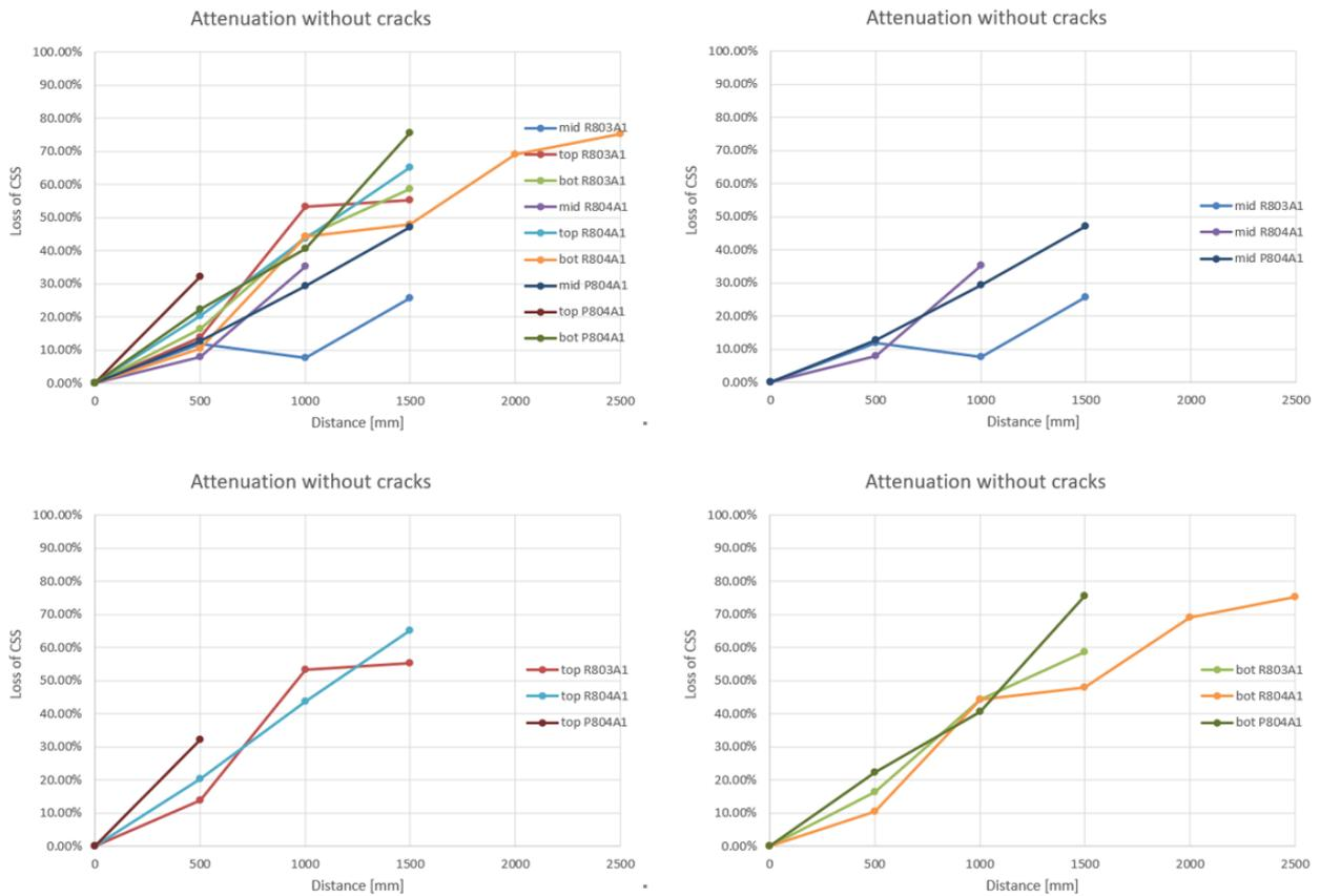
**Fig. 5.2.8 Attenuation of 800 mm beam in different layers (uncracked)**
