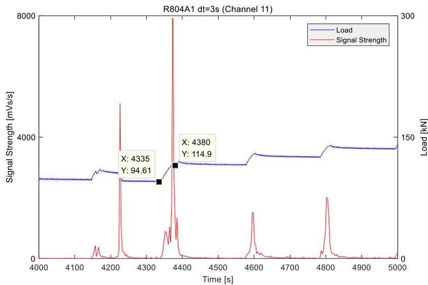
Fig. 5.2.13 Load and Signal strength against Time (R804A1 CHN11)
