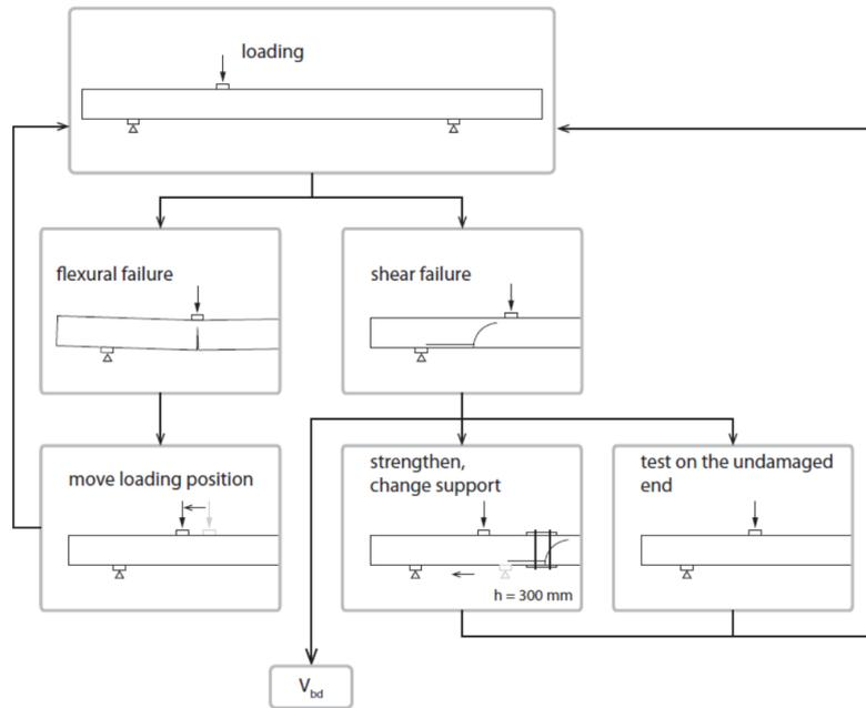
**Fig. 2.2.2** Flow chat of the test program for a given beam configuration
