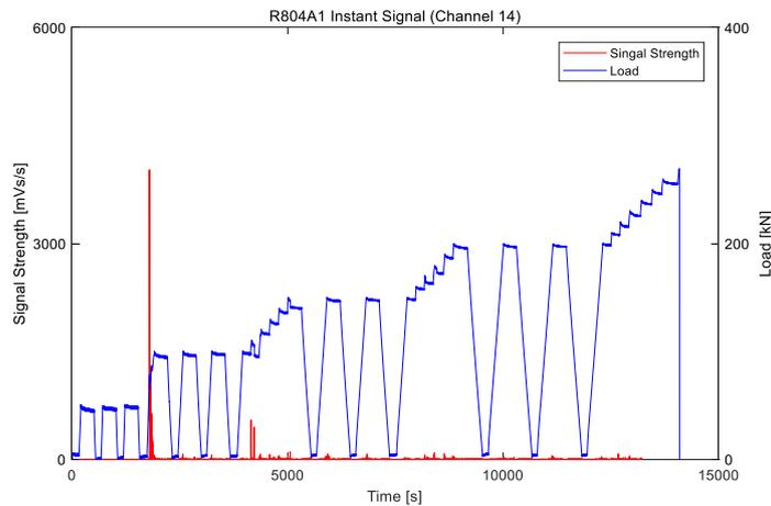
**Fig. 4.3.1 Load-time and SS-time curve of R804A1 (Channel 14 instant signal)**
