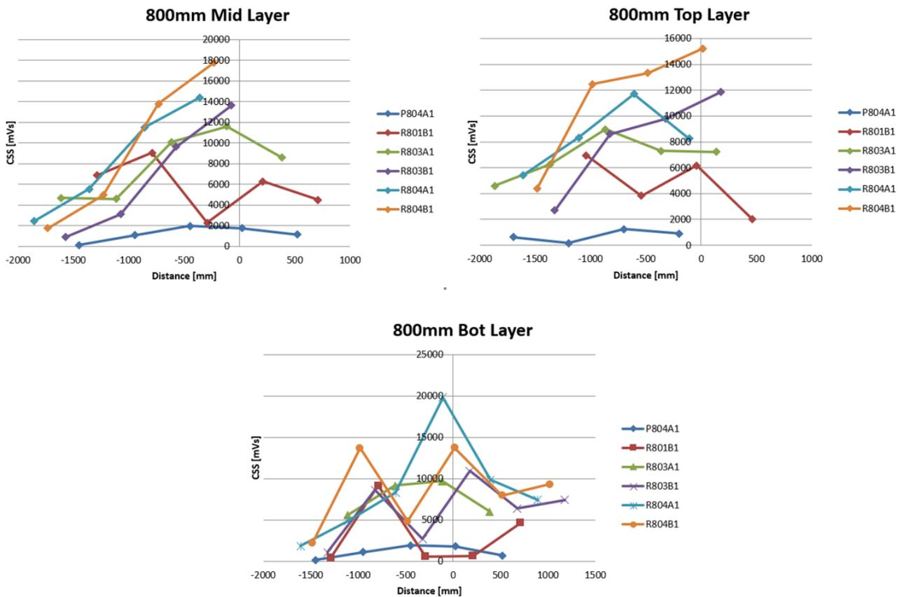
Fig. 5.2.15 CSS of 800 mm beam in different layers (cracked)
