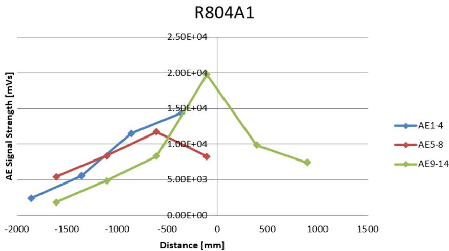
Fig. 5.2.14 CCS-Distance R804A1 (cracked)
