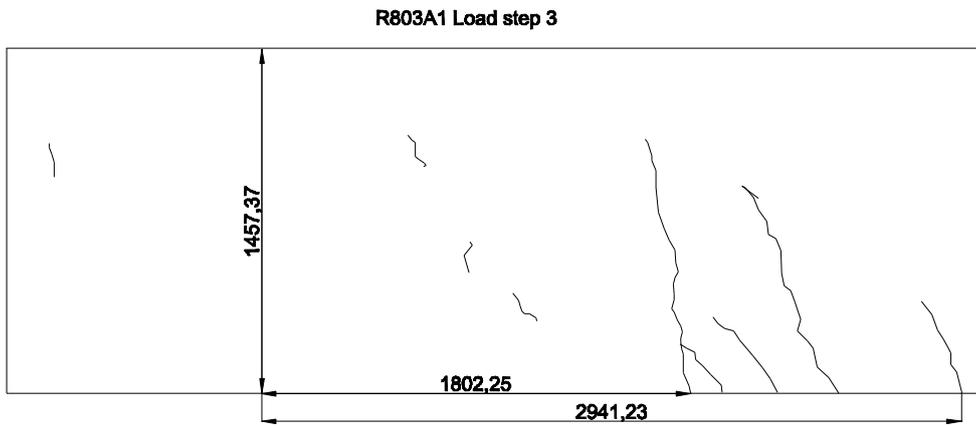
Fig.A3. 5 Crack pattern of load step 3
