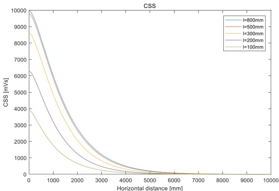
**Fig. 5.1.3 CSS versus Horizontal distance (different crack length)**
