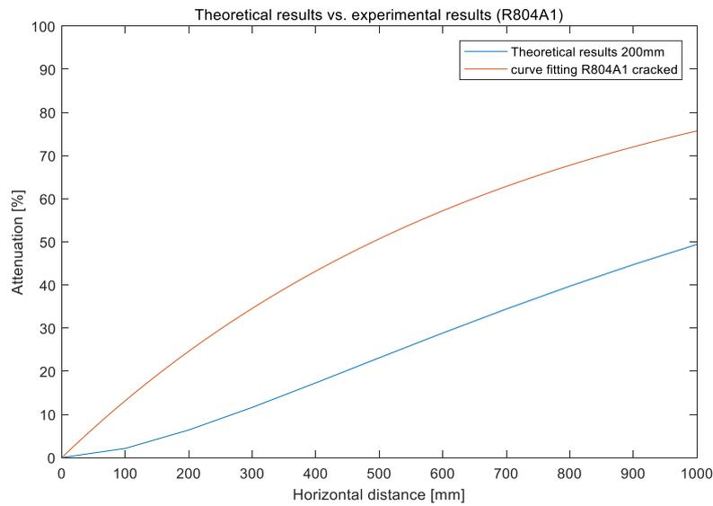
**Fig. 5.4.4 Theoretical results vs. experimental results (R804A1 cracked)**
