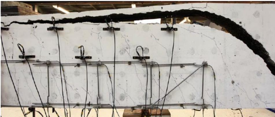
**Fig. 2.2.6 AE and LVDT grid**
