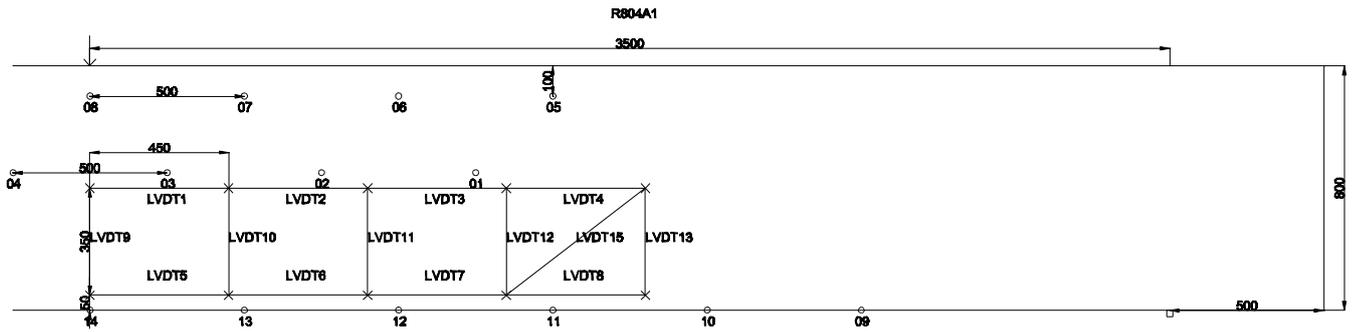
Fig. 3.3.1 AE layout of R804A1
