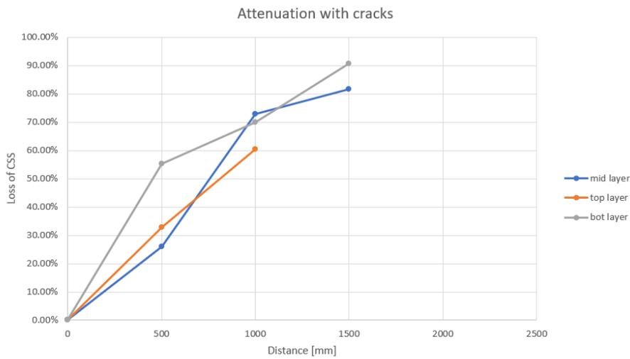
Fig. 5.2.17 Averaged attenuation of 800 mm beam in different layers (cracked)
