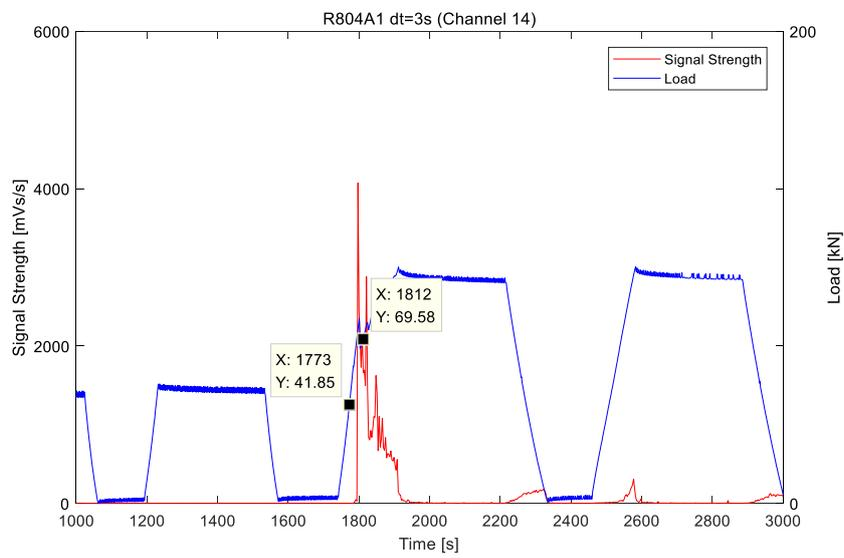
Fig. 5.2.5 SS-time curve of R804A1
