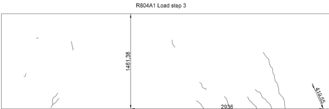
Fig. 5.4.2 Crack pattern of R804A1 load step 3
