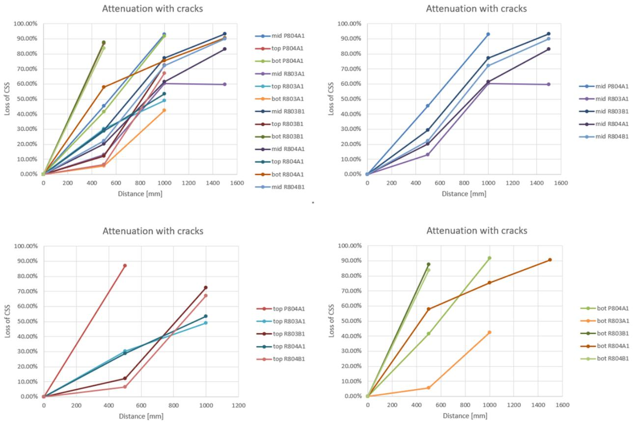
Fig. 5.2.16 Attenuation of 800 mm beam in different layers (cracked)
