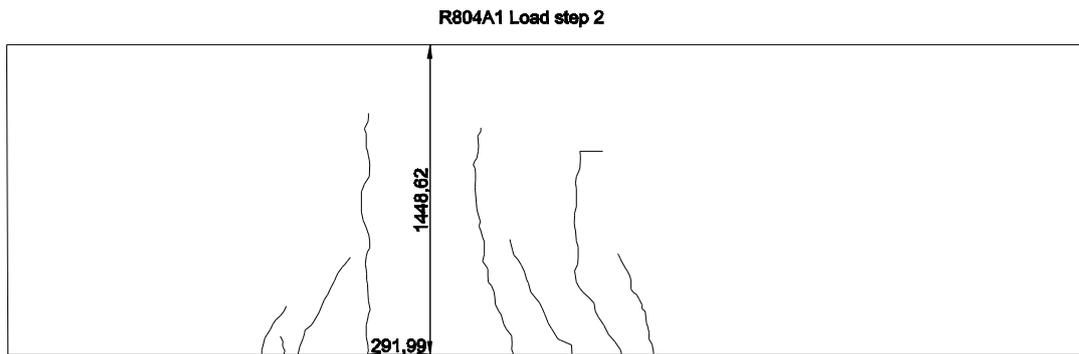
Fig. 5.2.4 Crack pattern of R804A1 load step 2
