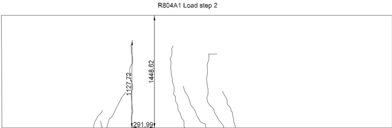
Fig. 5.4.1 rack pattern of R804A1 load step 2
