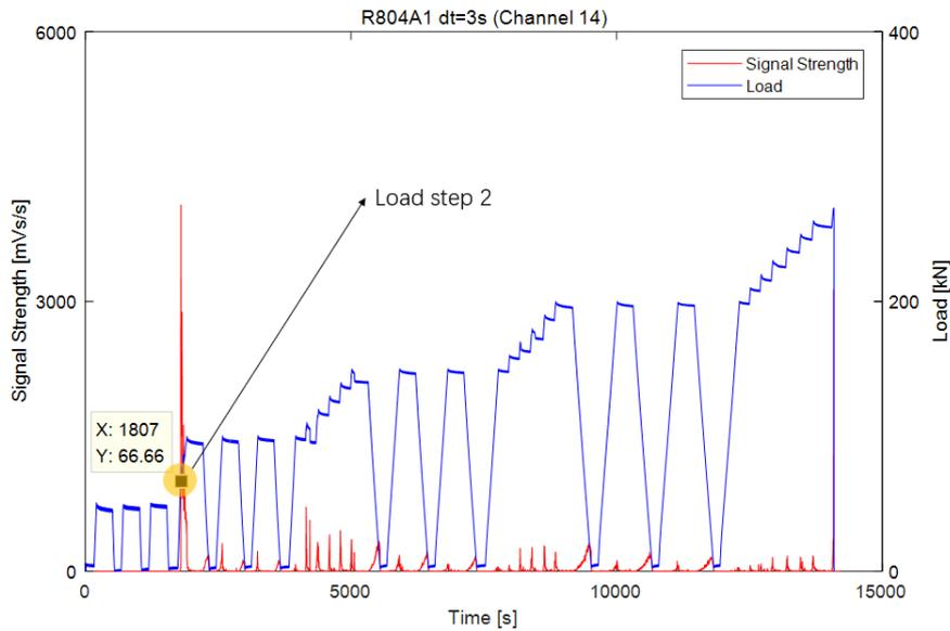
**Fig. 5.2.3 Load and Signal strength against Time (R804A1 CHN14)**
