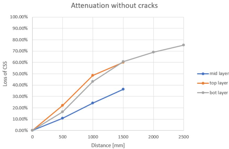
**Fig. 5.2.9 Averaged attenuation of 800 mm beam in different layers (uncracked)**
