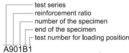
Fig. 2.1.1 Definition of test numbers in 1st stage
