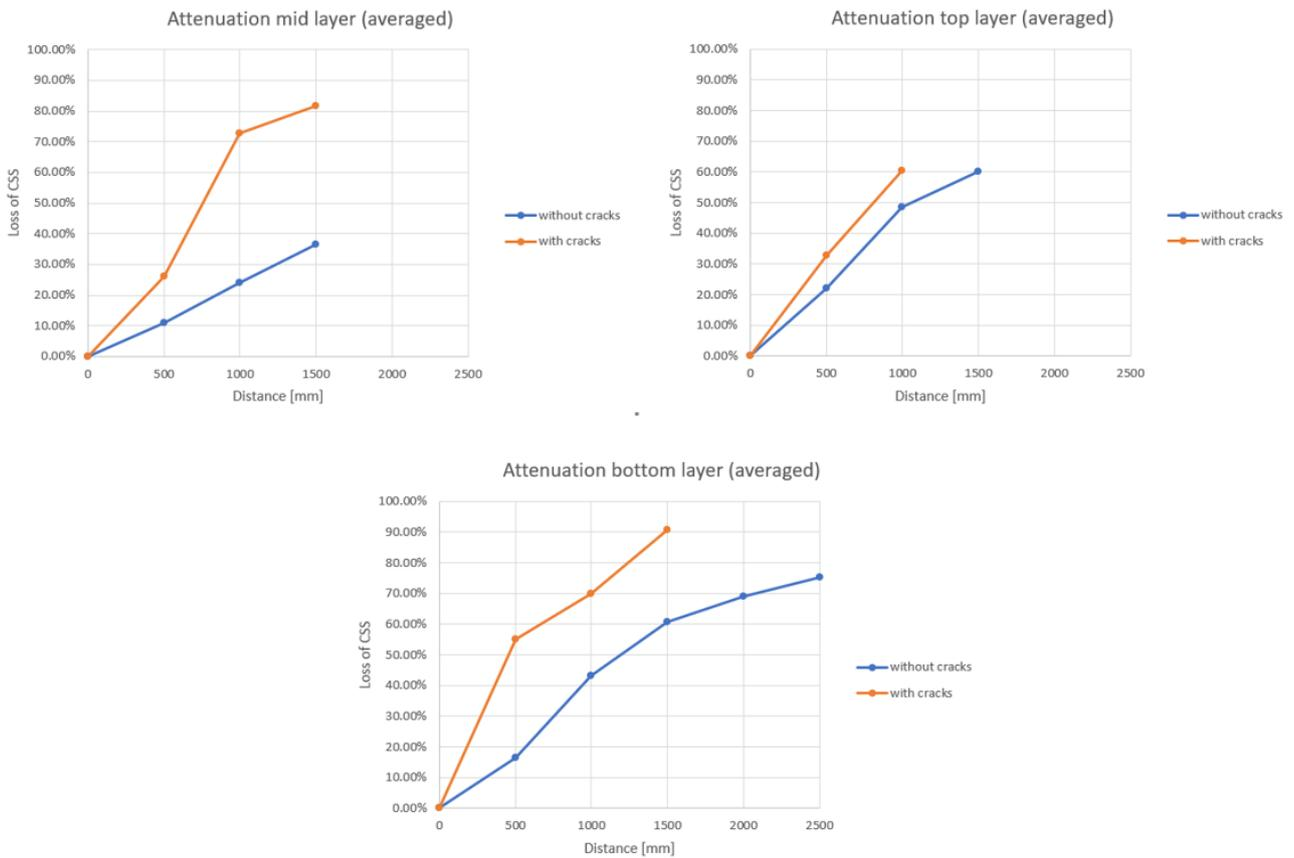
Fig. 5.3.1 Attenuation in cracked and uncracked structures
