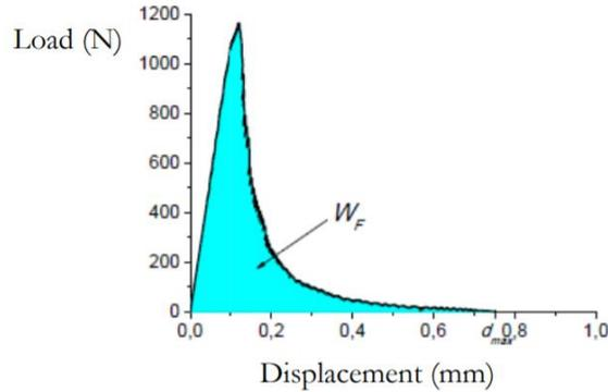
**Fig. 3.1.1 Load-displacement curve of concrete specimens**
