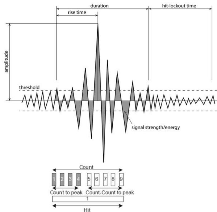
**Fig. 2.2.4 Conventional AE signal features**
