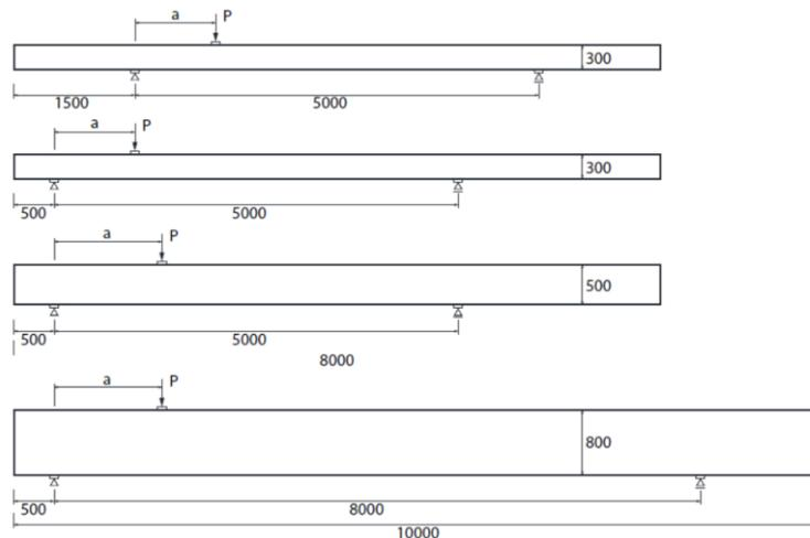
**Fig. 2.2.1 Configurations of the boundary conditions of the tests**
