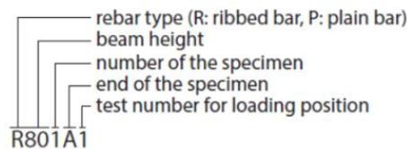
Fig. 2.1.2 Definition of test numbers in 2<sup>nd</sup> and 3<sup>rd</sup> stage
