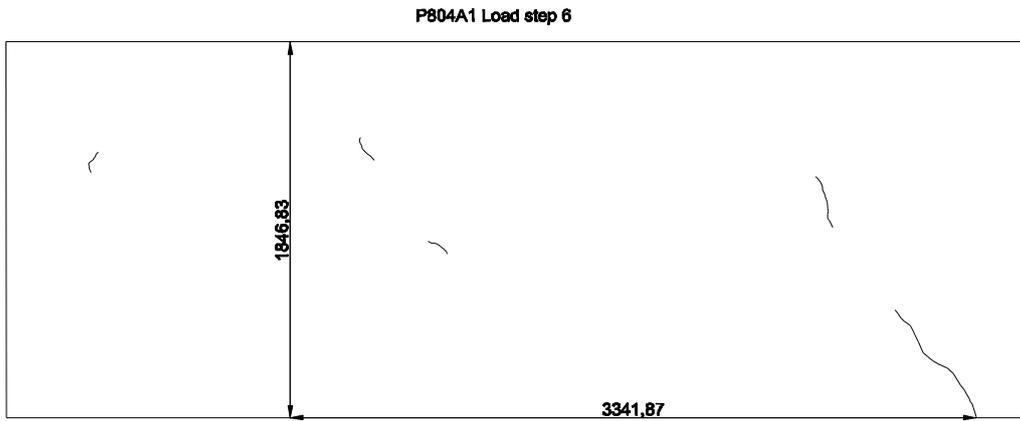
Fig.A3. 8 Crack pattern of load step 6
