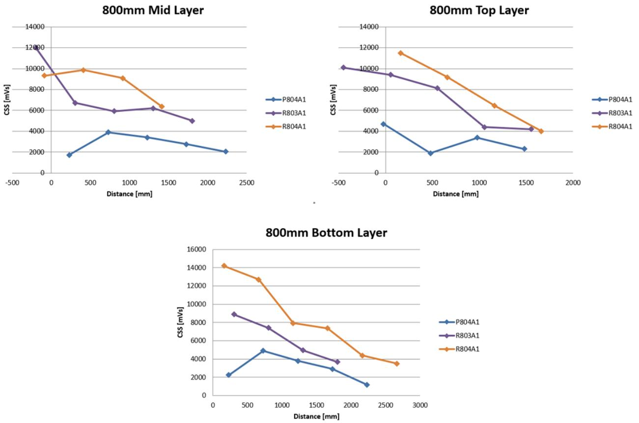
Fig. 5.2.7 CSS of 800 mm beam in different layers (uncracked)
