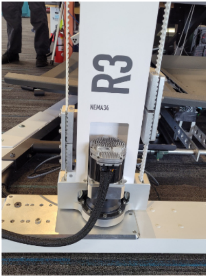
The actuated vertical mast
