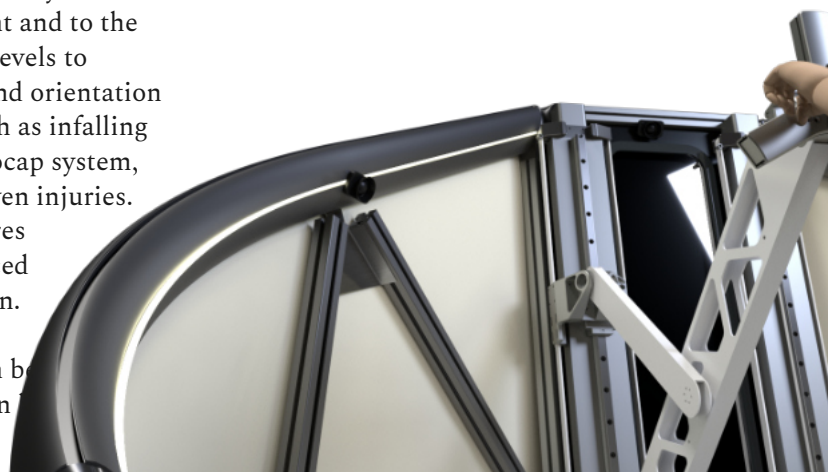
Close-up of LED strip in extrusion
