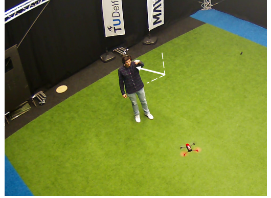
Fig. 25 Passive game mode 2: The user initiates a diagonal motion with the left hand
