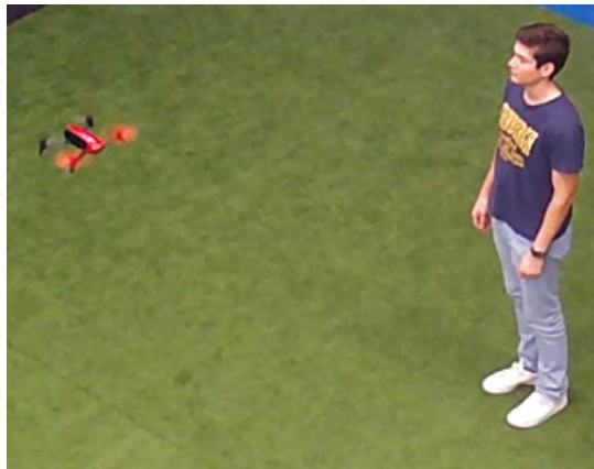
Figure 5.2: Stand By game mode before centering: the drone is trying to find the human user's facebox by rotating around a fixed axis
