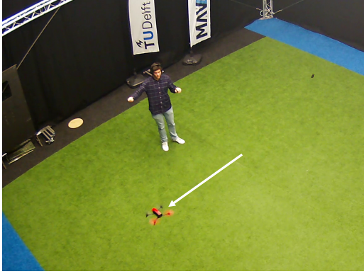
Fig. 24 Passive game mode Mode 2: The SAD mimics (a scaled version of) the user's hand motion
