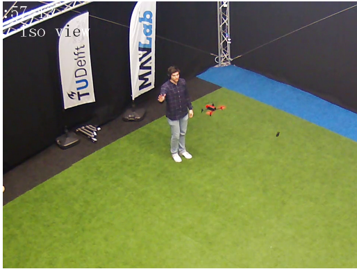
Fig. 32 Active game mode 4: The SAD moves to the right-hand side of the user and waits for the user's right hand to mirror this motion
