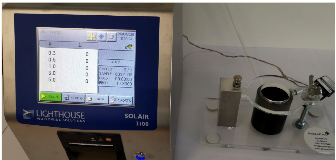
Fig 2. Lighthouse Solair 3100 particle counter connected to a particle chamber. When very dense filter materials are used with a very high PFE for the smallest particles, it causes a breathing resistance for the user [16, 17]. This resistance causes a pressure drop which was measured using an analog differential pressure sensor, type SDP2000-L (Sensirion AG, Staefa ZH, Switzerland) connected to the particle chamber. The pressure sensor is temperature compensated, calibrated and has a resolution of 11 Pa with a repeatability of 0.3% and accuracy of 1% [17]. The breathability requirements for respiratory protective devices are provided in a European standard [18]. The maximum permitted resistance (mbar) differs for the FFP1, FFP2, and FFP3 masks, ranging from 0.6–1.0 for inhalation at 30 l/min, 2.1–3.0 for 95 l/min and 3.0 for exhalation at 160 l/m. The norm for a FFP2-mask at 30 l/min is 0.7 mbar.
