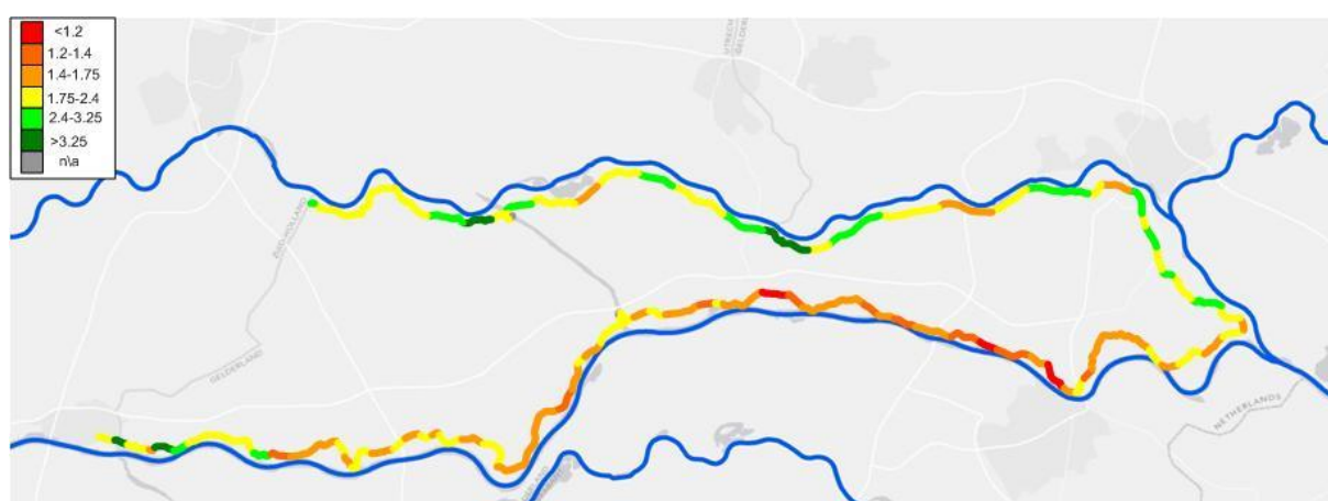
Figure A-3: Reduction factor of total flood probability according to FloRis (Van Rooijen, 2014)
