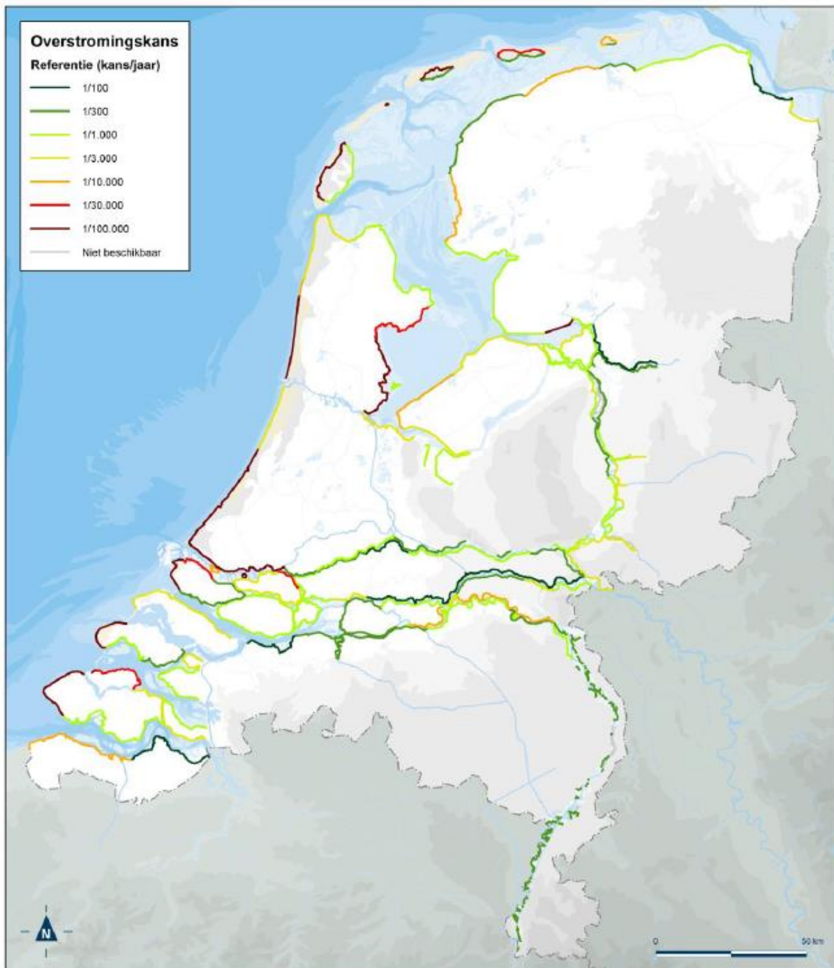
Figure A-11: Probability of flooding in the reference situation (Werkgroep Deelprogramma Veiligheid, 2014)
