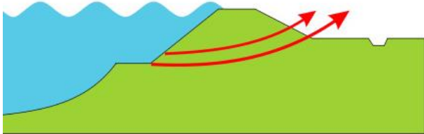
Figure 2-3: Failure mechanism piping and heave (Vergouwe, et al., 2014)
