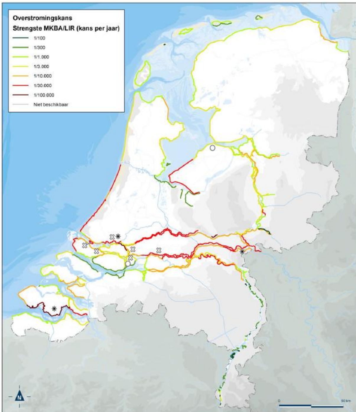
Figure A-17: Combined probability of flooding standard (Werkgroep Deelprogramma Veiligheid, 2014)
