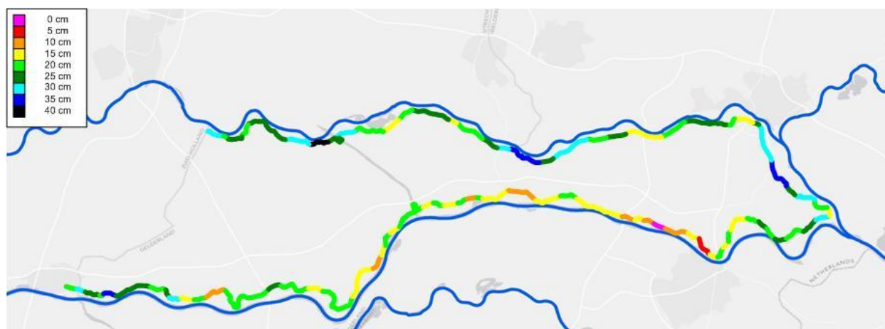
Figure A-2: water level reduction due to RfR according to FloRis (Van Rooijen, 2014)
