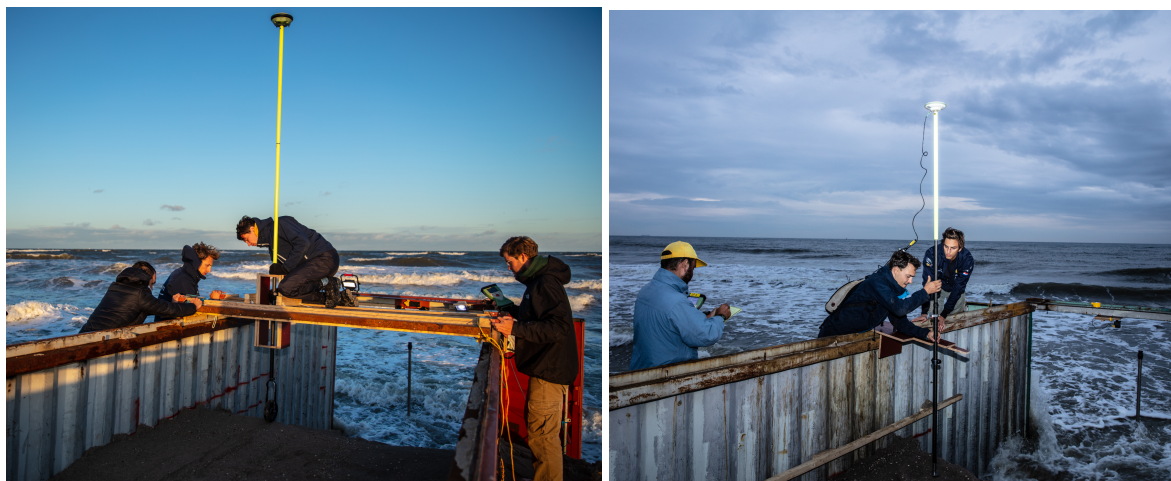
(a) GPS setup container 1. A cart on top of the container with a frame attached to it can guide a GPS pole through the container. This way transects of the dune face are taken.
