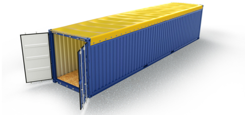
Figure 2.1: 3D overview of an open-top shipping container with a yellow sail on top. This container is used as a contained dune erosion environment.
