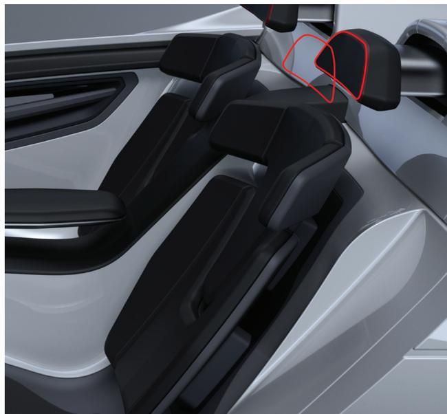
FIGURE 6.5 Misplaced headrest
