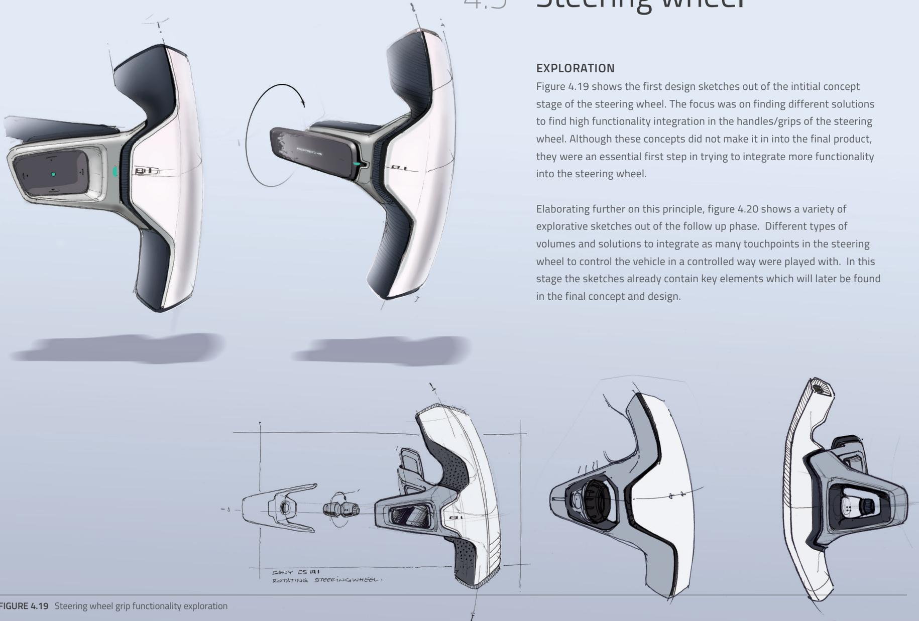
FIGURE 4.19 Steering wheel grip functionality exploration
