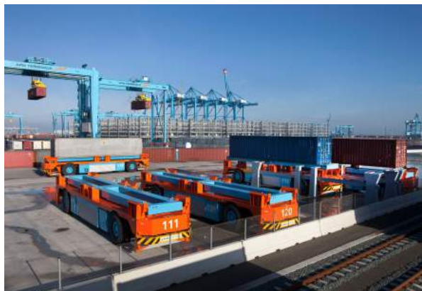
(a) AGVs at the APM terminal, Maasvlakte 2, Netherlands.
