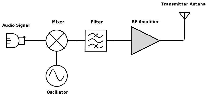
Figure 1.1: A basic overview of a transmitter system.
