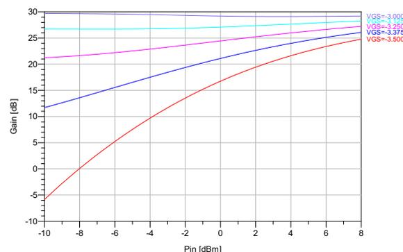
Figure 4.5: When sweeping  $V_{GS}$  different linearity characteristics can be achieved. These simulations have been performed with  $V_{DD} = 31.6$  V on a single transistor stage
