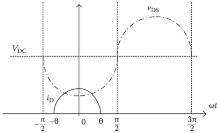
Figure 3.6:  $V_{DS}$  and  $I_D$  waveforms for class C PA. [13]
