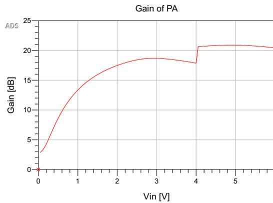
Figure 4.26: Effect on the Gain by lowering  $V_{GS,main}$ .
