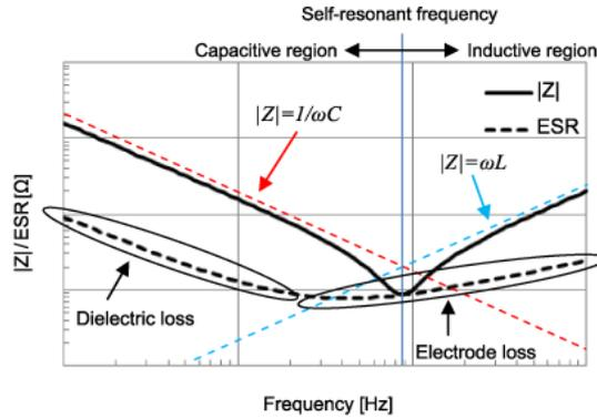
Figure 4.13: Capacitive and inductive regions of a non-ideal capacitor [19].
