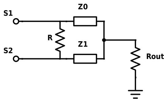
Figure 4.17: Simple configuration of a Wilkinson Power Combiner
