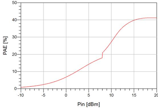
Figure 4.3: The PAE when biasing the transistor in class A
