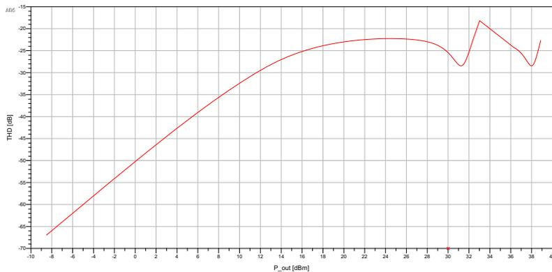
Figure 4.29: Total Harmonic Distortion of the system.
