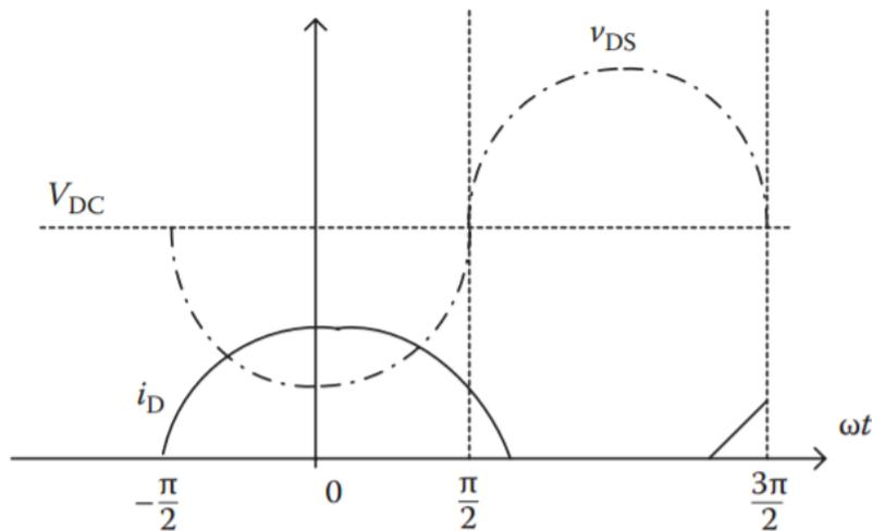
Figure 3.5:  $V_{DS}$  and  $I_D$  waveforms for class AB PA. [13]
