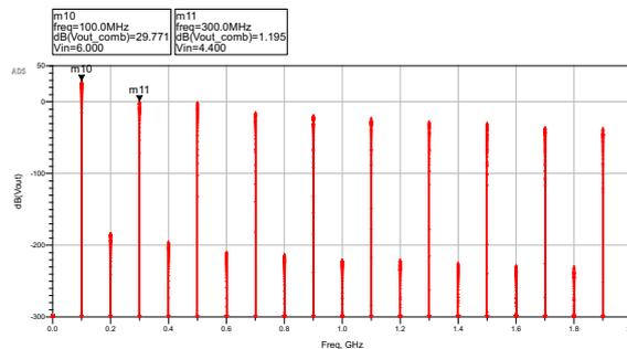
Figure 4.11: Frequency components of the output signal with  $\lambda/4$  line added.
