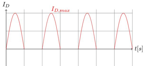
Figure 4.1: Drain current for transistor biased in class B.
