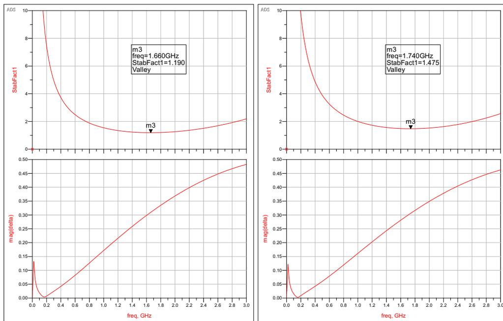
(a) Rollet factor and  $\Delta$  for  $V_{DD} = 14$  V
