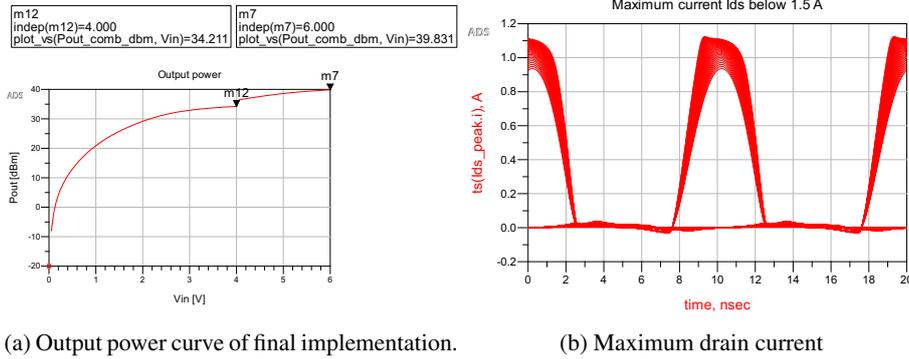
(a) Output power curve of final implementation. (b) Maximum drain current
