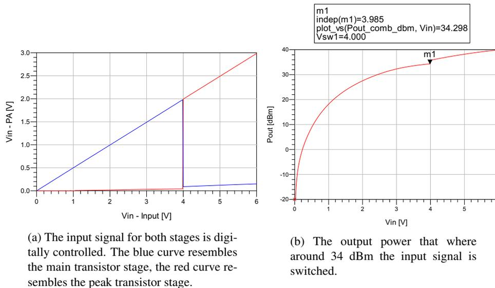
Figure 4.14: Switching profiles for a switching point of 4 V.
