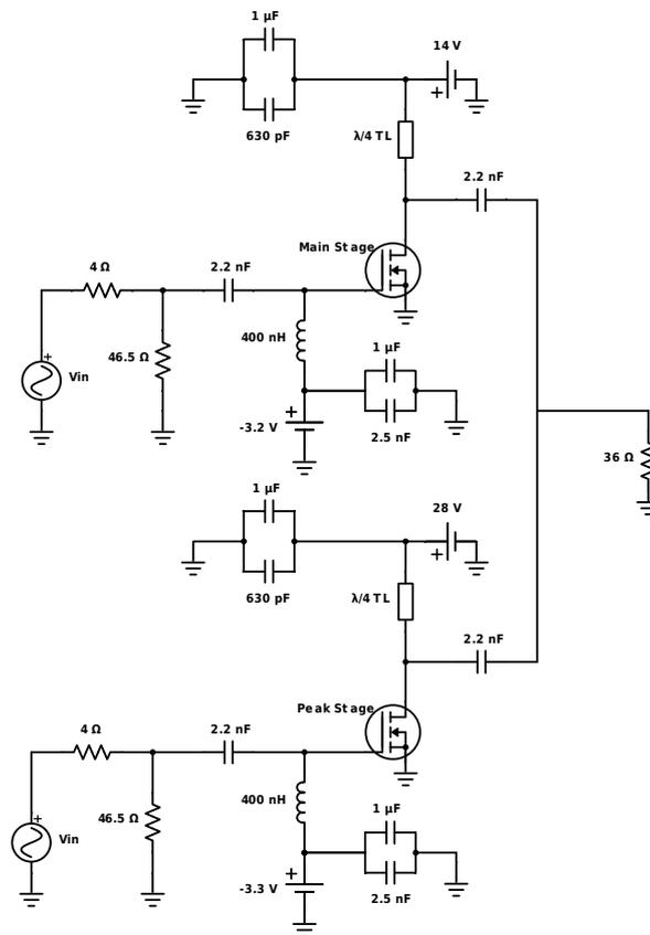
Figure 4.23: PA circuit that is designed for RF Application
