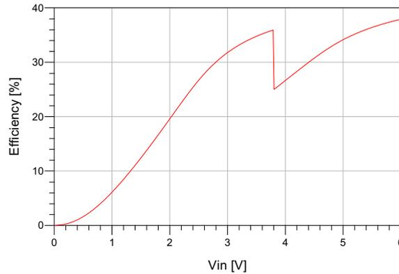
Figure 4.19: Drain efficiency when using a Wilkinson Power Combiner
