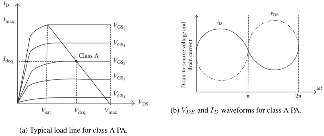
Figure 3.3: Class A power amplifier characteristics. [13]
