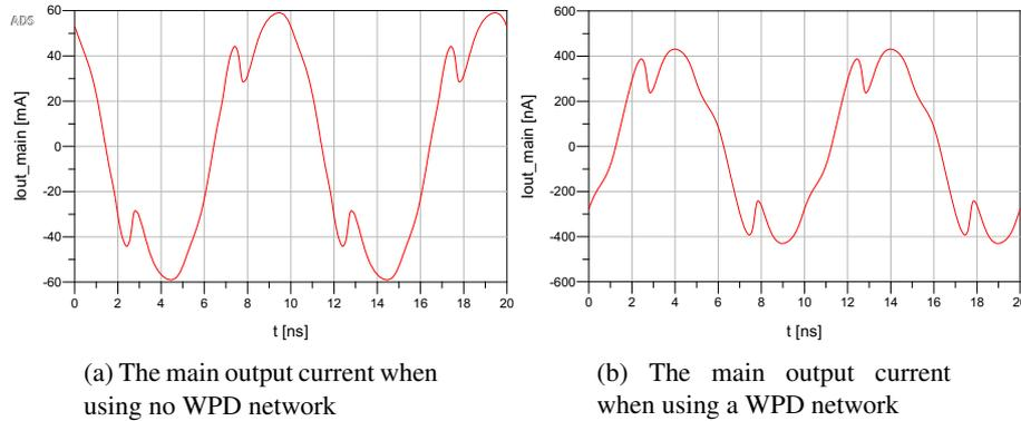
Figure 4.18: The different output current profiles. Be aware of the difference in magnitude.
