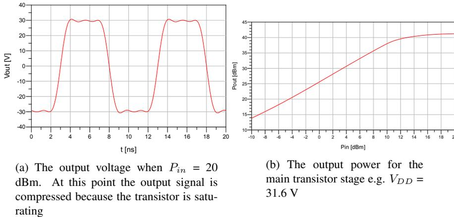
Figure 4.8: Harmonics effecting the signal at the output of the amplifier resulting in a higher output power than calculated
