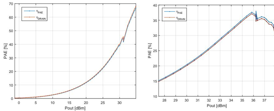
(a) Measured efficiency of the main amplifier. (b) Measured efficiency of the peak amplifier.
