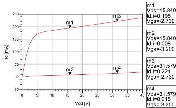
Figure 4.6: Simulations verify that a different quiescent current is obtained when biasing in different classes
