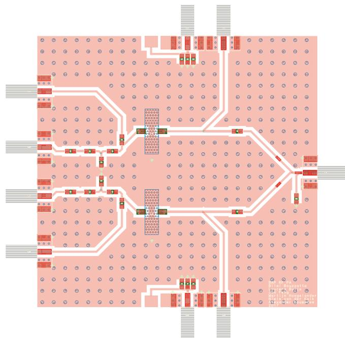
Figure 4.31: Final PCB layout.
