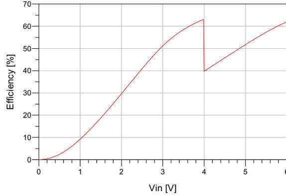
Figure 4.15: The efficiency profile when using direct switching.
