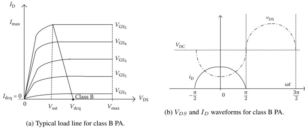
Figure 3.4: Class B power amplifier characteristics. [13]
