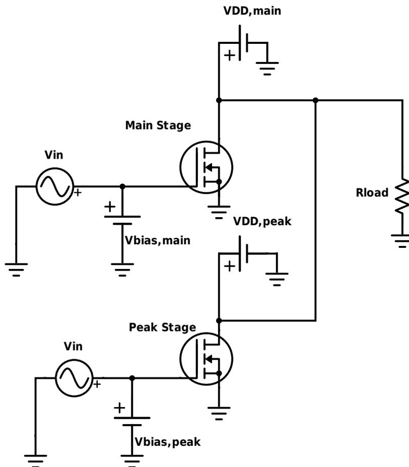
Figure 1.3: A basic overview of the supply interpolating power amplifier
