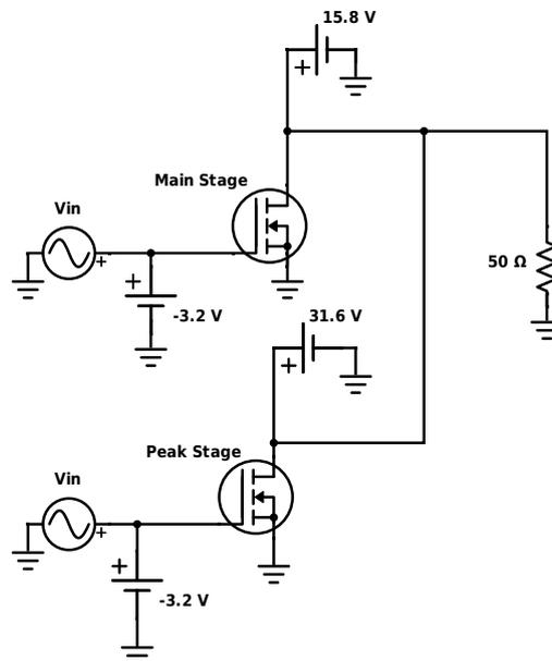
Figure 4.7: First circuit obtained by DC analysis of the transistor. This circuit is of course never applicable to RF signals.
