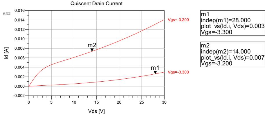
Figure 5.2: Quiescent drain current bias in the variable gain interpolating supply amplifier.
