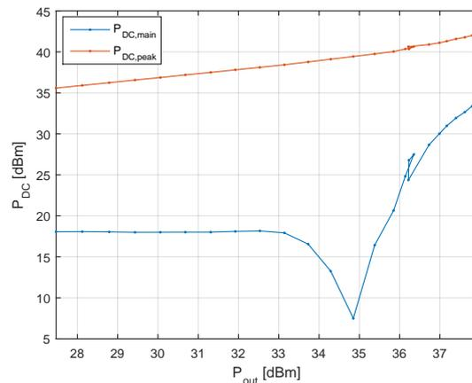
Figure 5.4: DC power consumption in the peak amplifier stage.
