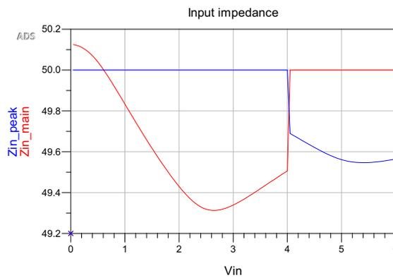
Figure 4.27: Input impedances of the main and peak amplifiers.
