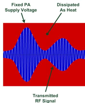
Figure 1.2: Using a fixed power supply voltage, a lot of power can be dissipated as heat
