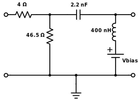
Figure 4.20: The circuit that has been designed to improve stability
