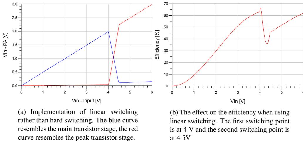
Figure 4.16: Characteristics of linear switching
