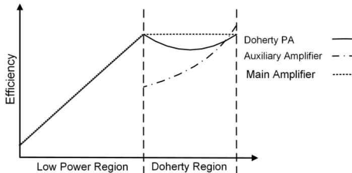
Figure 3.8: Doherty Power Amplifier efficiency curve.
