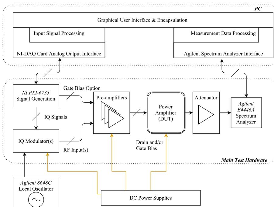
Figure 5.1: Test setup used throughout the measurement phase of the project.
