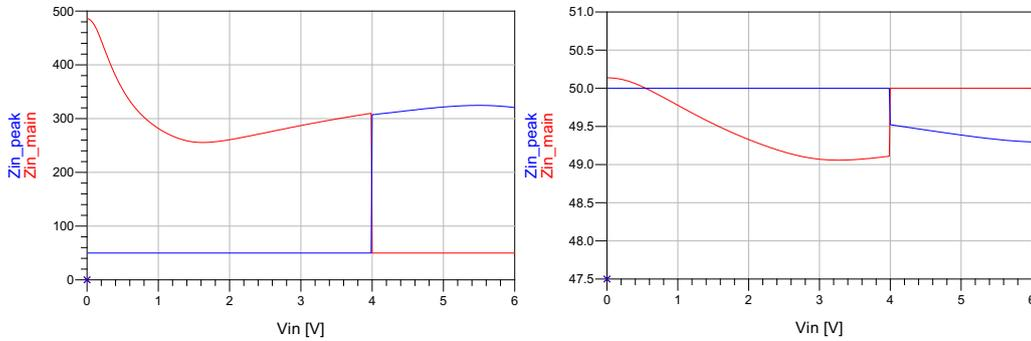
Figure 4.12: On the left: input impedance without matching resistor. On the right: input impedance with matching resistor. The red curves indicate the input impedance for the main transistor stage, the blue curves indicate the input impedance for the peak transistor stage
