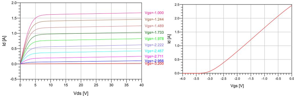
(a) Plot of  $I_D$  vs  $V_{DS}$  curvatures for different values of  $V_{GS}$  (b) Plot of  $I_D$  vs  $V_{GS}$  from where it can be seen that  $V_{TH} \approx -3.3$  V
