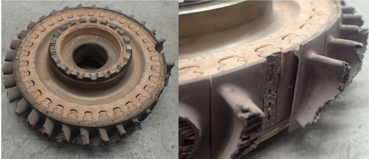
**Figure 2.4:** First stage turbine rotor of a 331-500 after T1 blade failure showing extensive impact damage.
