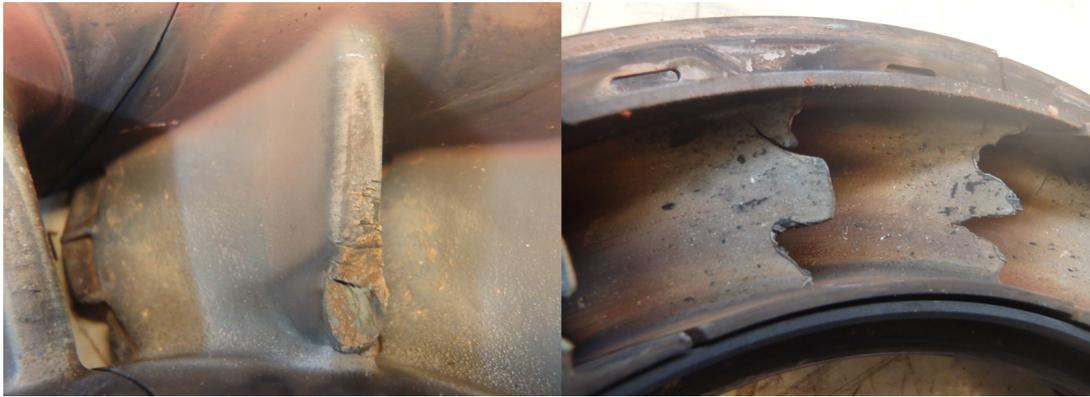
**Figure 8.10:** Deterioration in the first stage NGV of APU 1925 after removal due to high time.
