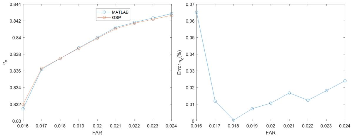
**Figure 4.9:** Comparison in compressor isentropic efficiency between the MATLAB and GSP models.
