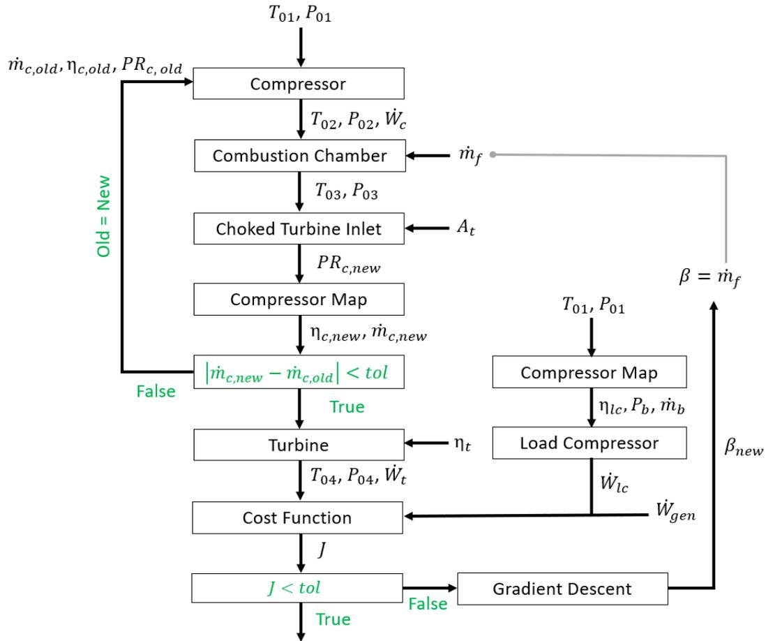
**Figure 6.3:** Calculation process for generating deterioration data using the WBM. The fuel flow is adjusted until a net-zero work balance on the shaft is achieved.
