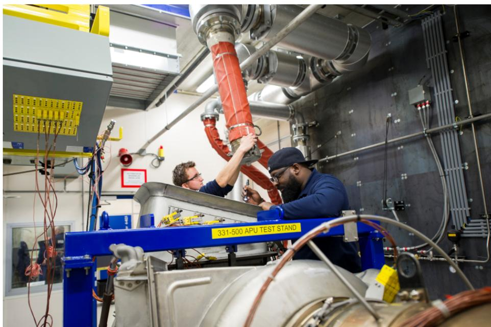
**Figure 1.5:** The preparation of a Honeywell 331-50 APU for testing at EPCOR.
