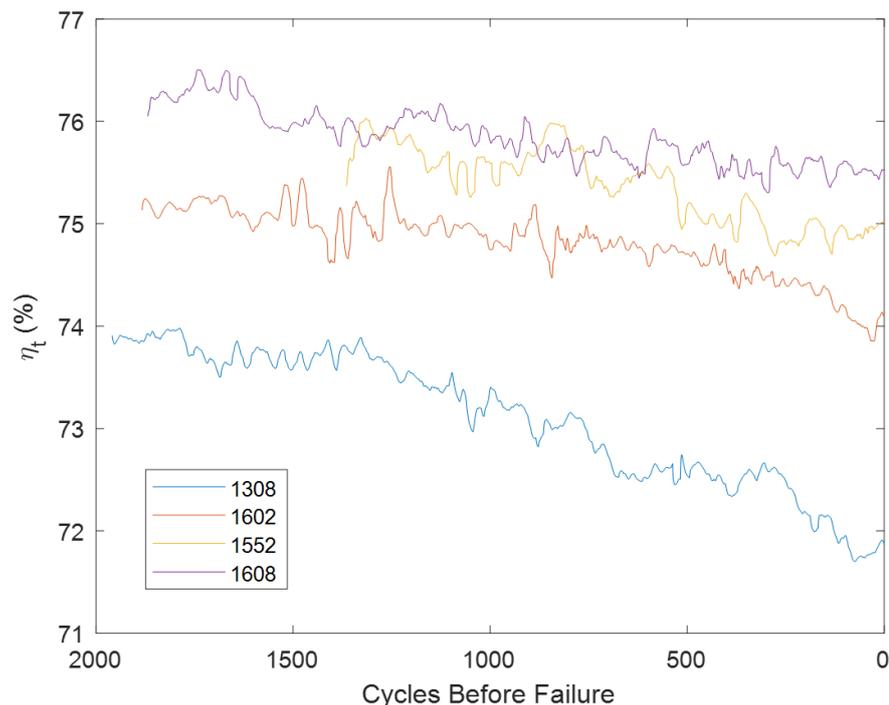
**Figure 8.1:** Deterioration in turbine efficiency for four 331-500 APUs in the lead-up to failure.
