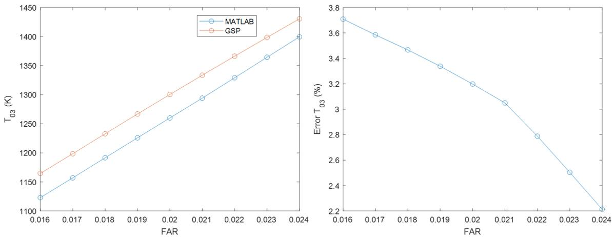
**Figure 4.10:** Comparison in TIT between the MATLAB and GSP models.
