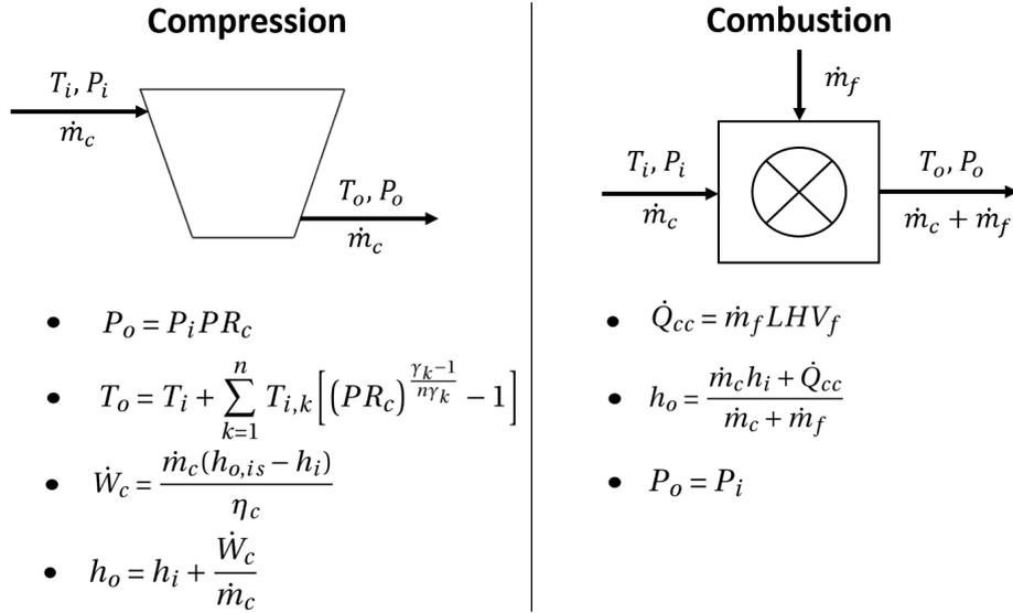
**Figure 4.2:** Equations used for the compression and combustion processes of the thermodynamic model.
