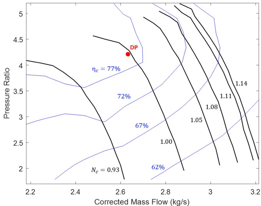
**Figure 6.2:** Assumed compressor map for the load compressor of the Honeywell 331-500 APU as scaled from the *smallhpc* map from GSP.
