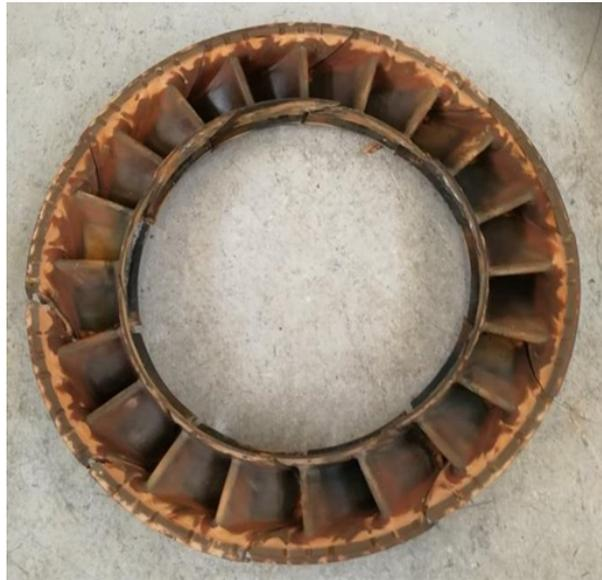
**Figure 5.5:** Assembled first stage NGV of the Honeywell 331-500 APU.
