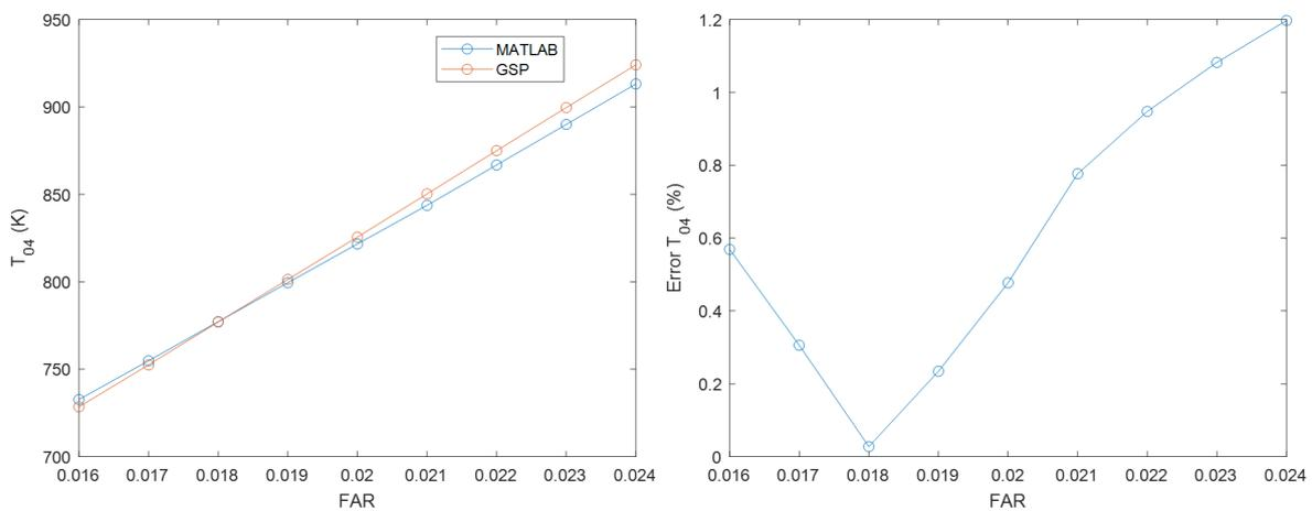
**Figure 4.11:** Comparison in EGT between the MATLAB and GSP models.
