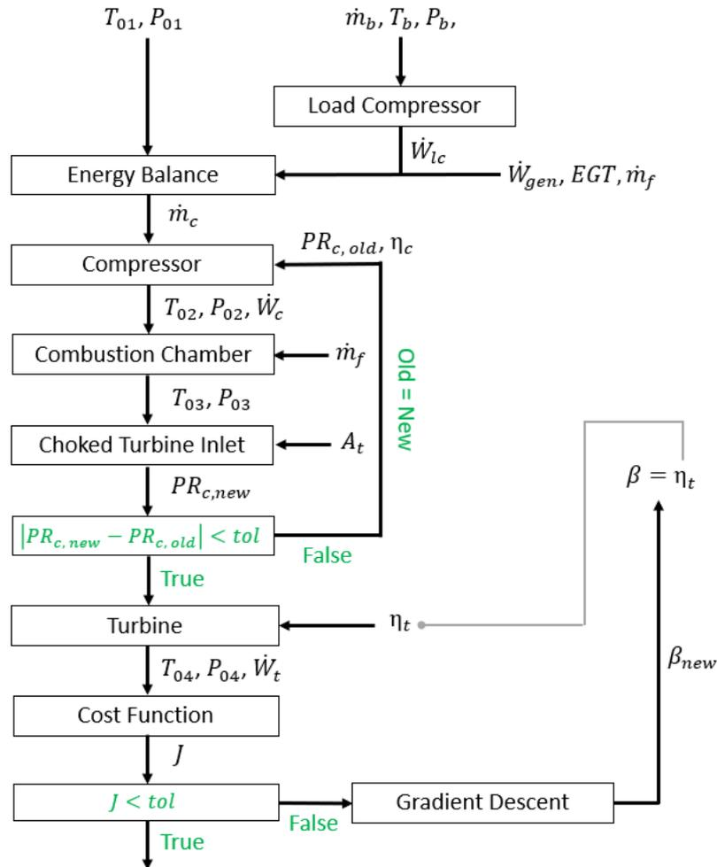
**Figure 5.7:** Calculation process for fitting the BBM to the on-design operation of the 331-500. The turbine efficiency is adapted until the error between the calculated and measured EGT is minimised.
