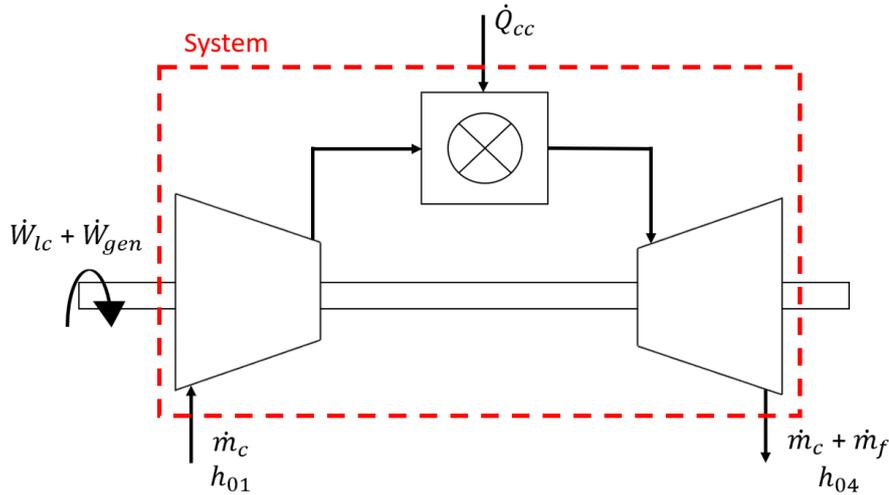
**Figure 5.4:** Definition of the system around the APU power section from which an energy balance is taken for estimating the compressor mass flow.
