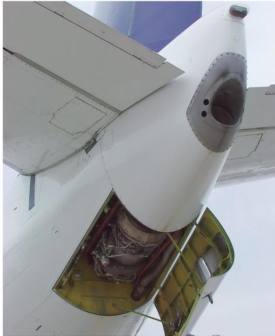
**Figure 1.1:** The tail of the Boeing 737-300 showing the APU and its exhaust outlet [4].
