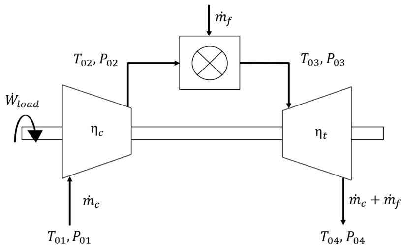
**Figure 4.1:** Schematic of the main components along the gas path of a single-shaft gas turbine.
