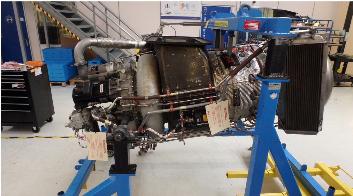
**Figure 5.1:** The Honeywell 331-500 APU in a stand at the shop floor of EPCOR B.V.
