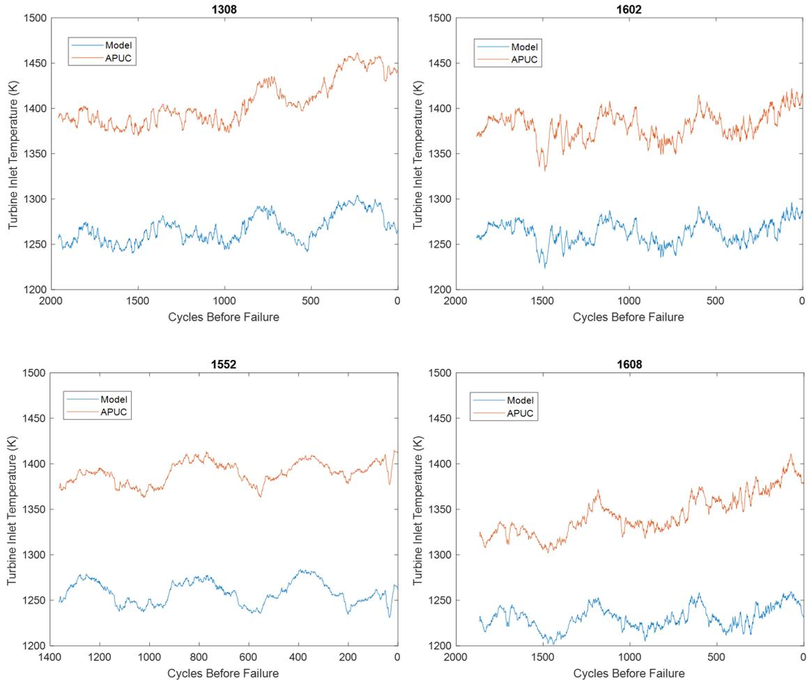
**Figure 8.3:** Comparison between model- and controller-calculated TIT data for APUs 1308, 1602 1552 and 1608 in the lead-up to T1 blade failure.
