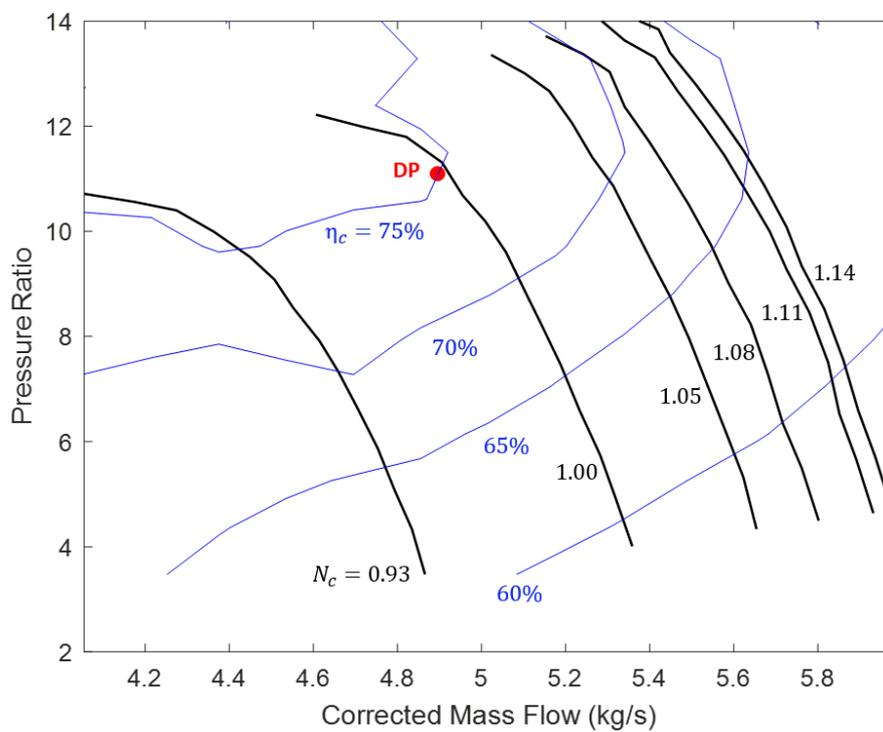
**Figure 6.1:** Assumed compressor map for the compressor of the Honeywell 331-500 APU as scaled from the *smallhpc* map from GSP.
