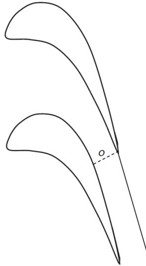
**Figure 4.4:** Definition of the throat as the distance  $O$  between two adjacent turbine stator vanes [14].
