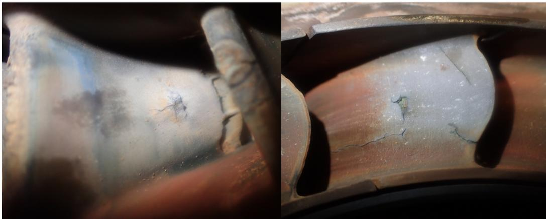
**Figure 8.9:** Deterioration in the first stage NGV of APU 1710 after removal due to high time.
