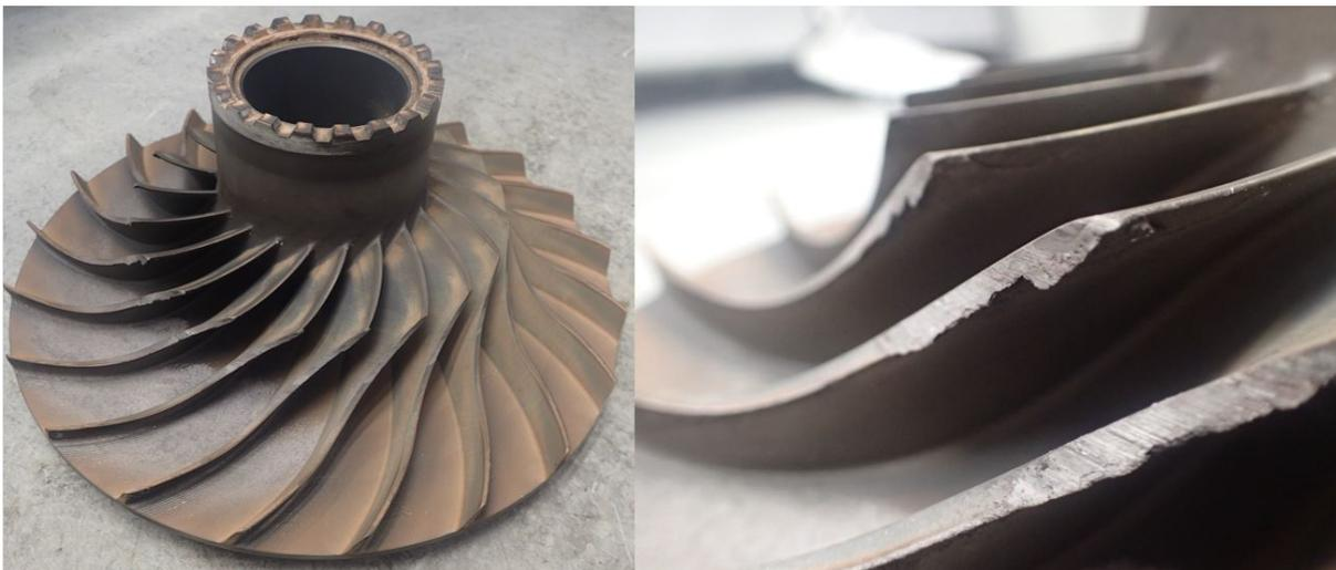
**Figure 2.7:** Second stage compressor impeller of the 331-500 after T1 blade failure showing heavy abrasion of the contours.
