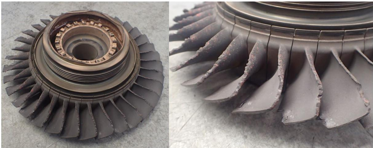
**Figure 2.5:** Second stage turbine rotor of a 331-500 after T1 blade failure showing extensive impact damage.
