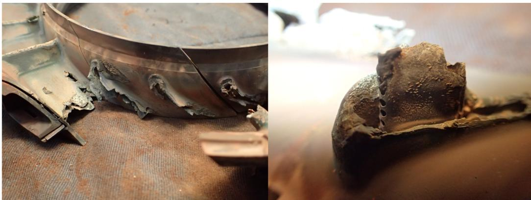
**Figure 8.16:** Deterioration in the first stage NGV of APU 1590 after removal due to high time.
