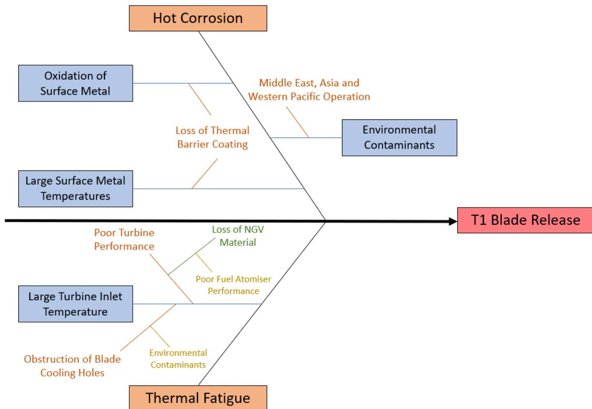
**Figure 2.1:** Cause-and-effect diagram of the potential factors that lead to a first stage turbine blade release on the Honeywell 331-500.
