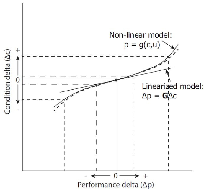
**Figure 3.1:** Effect of linearising the non-linear performance of a gas turbine about a single operating point [8].
