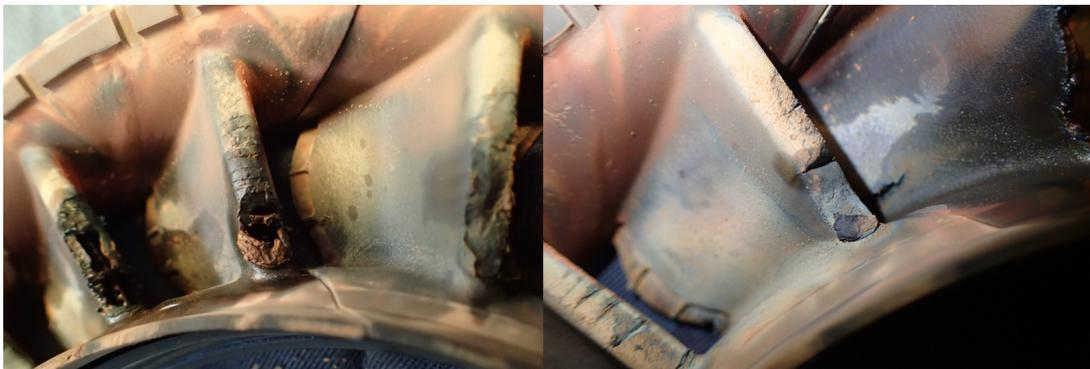
**Figure 8.11:** Deterioration in the first stage NGV of APU 1835 after removal due to high time.
