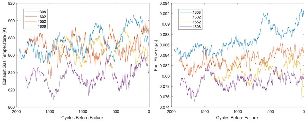
**Figure 8.2:** Measured EGT and fuel flow data for the four 331-500 APUs in the lead-up to T1 blade failure.
