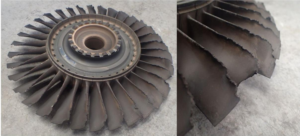
**Figure 2.6:** Third stage turbine rotor of a 331-500 after T1 blade failure showing extensive impact damage.
