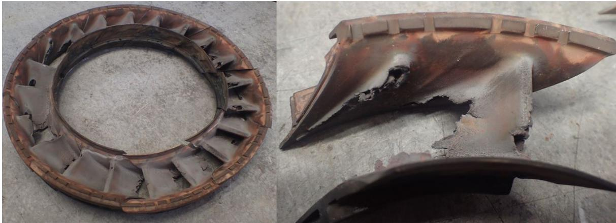
**Figure 2.2:** The first stage NGV assembly of the turbine of a 331-500 showing extensive corrosion and damage.
