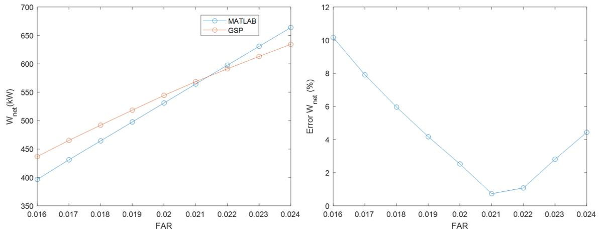
**Figure 4.12:** Comparison in net shaft work between the MATLAB and GSP models.
