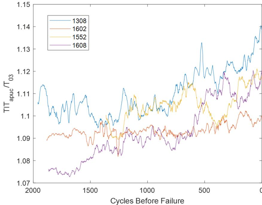
**Figure 8.4:** Ratio of controller- to model-calculated TIT for the four 331-500 APUs in the lead-up to T1 blade failure.
