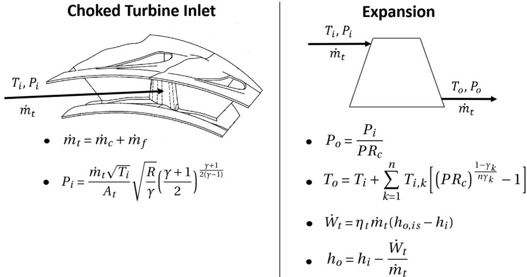
**Figure 4.3:** Equations used for the choking and expansion processes of the thermodynamic model.
