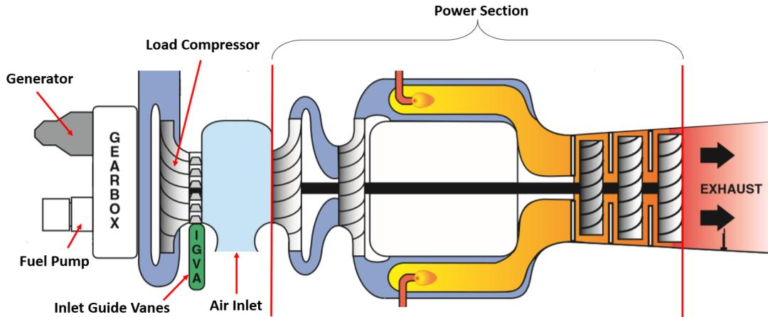
Figure 5.2: Diagram of basic components of the Honeywell 331-500 APU [15].
