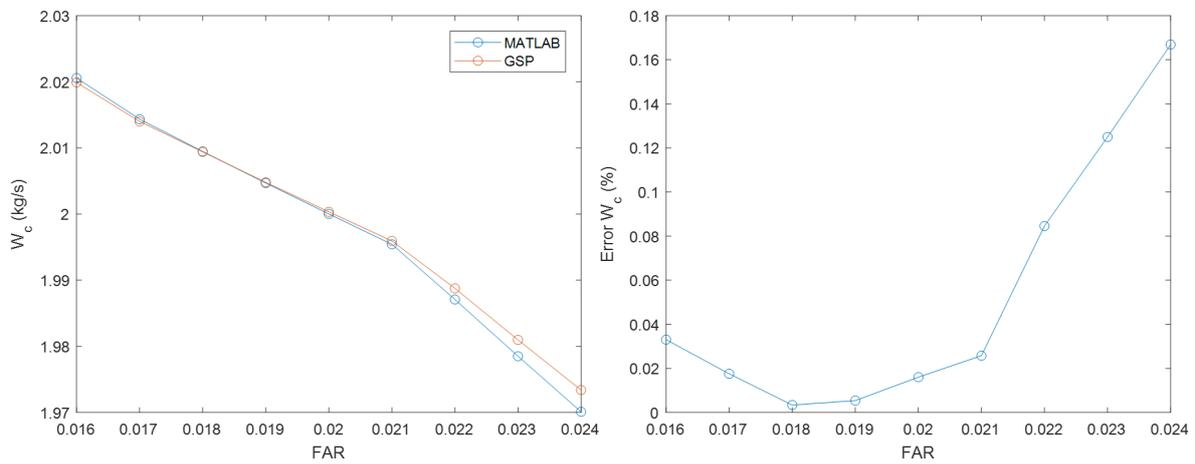
**Figure 4.7:** Comparison in corrected compressor mass flow between the MATLAB and GSP models.
