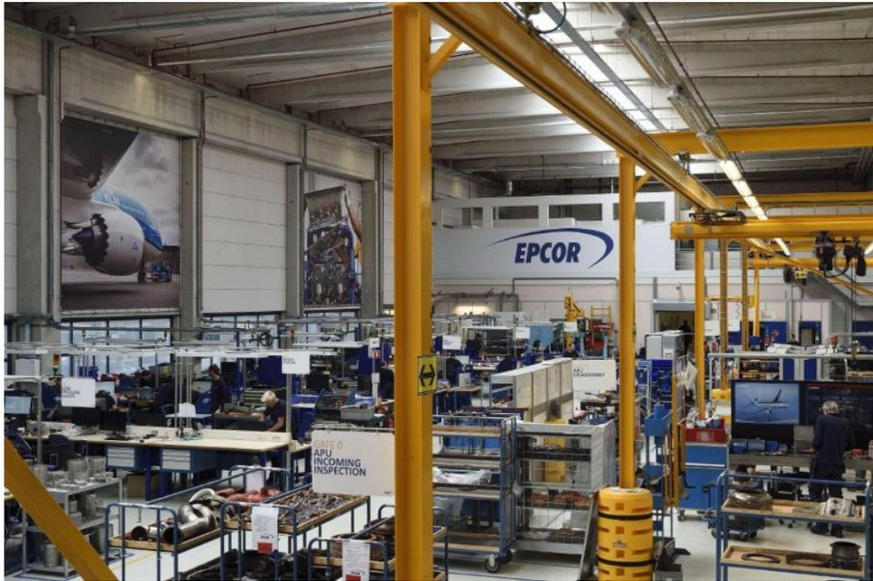
**Figure 1.3:** Shop floor at EPCOR where APUs and aircraft components undergo repair and overhaul.
