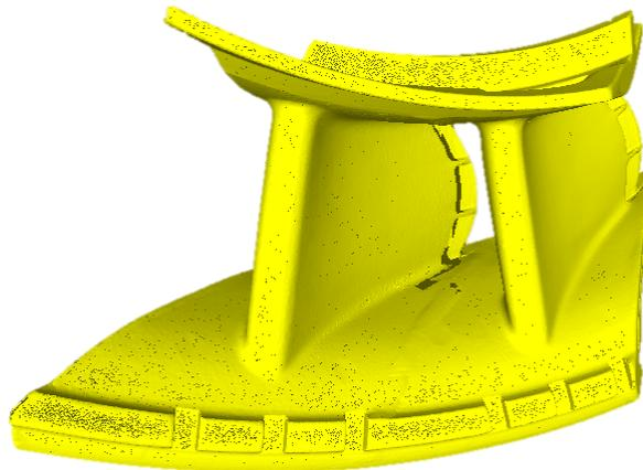
**Figure 5.6:** 3-D scan of a single nozzle segment from the first stage NGV of the Honeywell 331-500.
