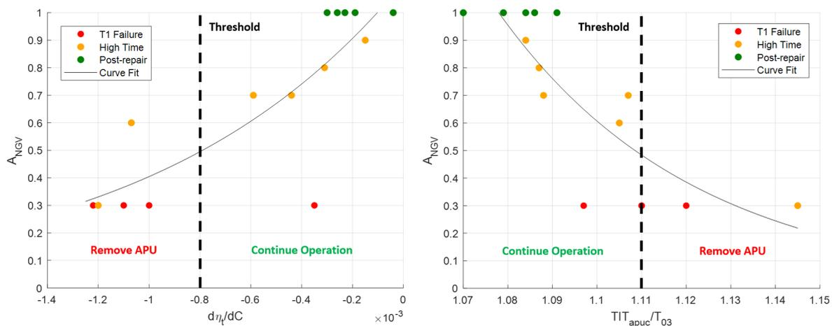
**Figure 9.1:** Definition of the threshold of  $-0.8 \times 10^{-3}$  and 1.11 on the turbine efficiency gradient and TIT ratio to signal a heavily deteriorated turbine of the Honeywell 331-500.
