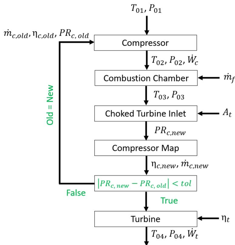
**Figure 4.6:** Calculation process for the off-design operation of a single-shaft gas turbine with a choked turbine inlet.
