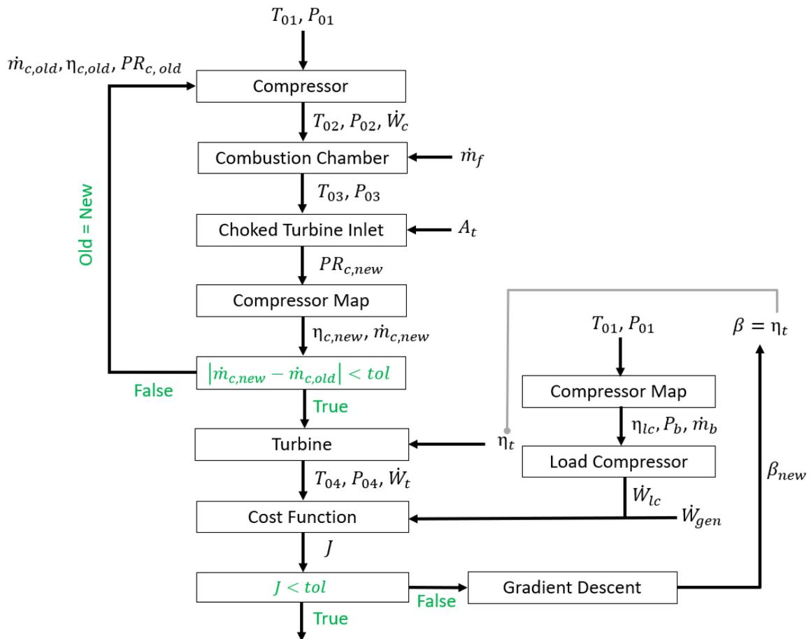
**Figure 6.4:** Calculation process for adapting the turbine efficiency to minimise the error between the 500TM and the generated performance data.
