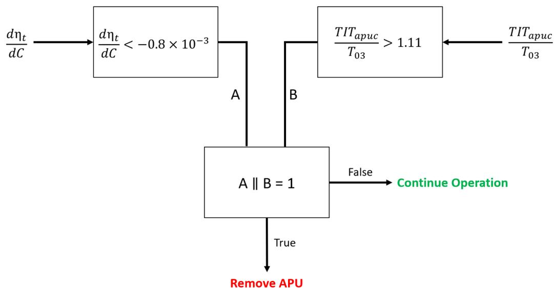
**Figure 9.2:** Visual representation of a rule functioning as a threshold on the turbine efficiency gradient and TIT ratio to signal the removal of a 331-500.
