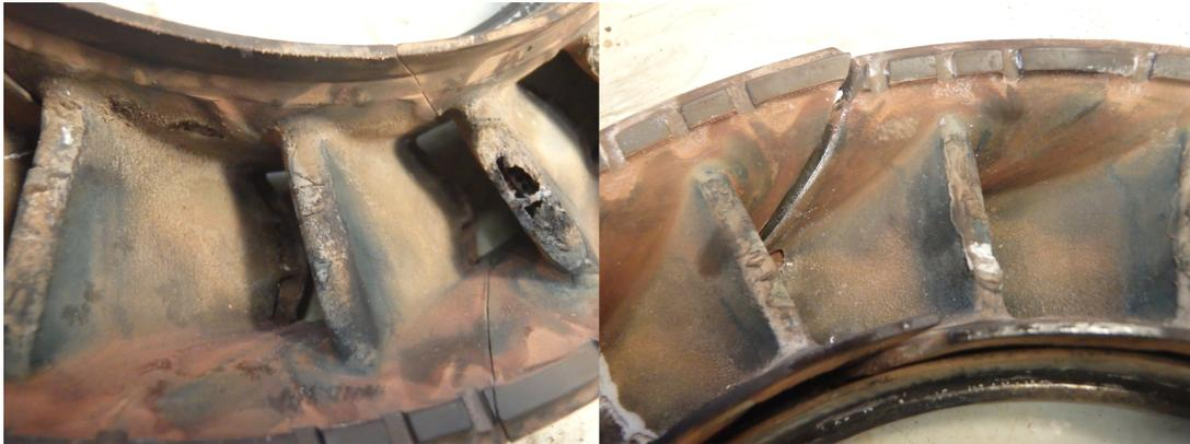
**Figure 8.13:** Deterioration in the first stage NGV of APU 1466 after removal due to high time.
