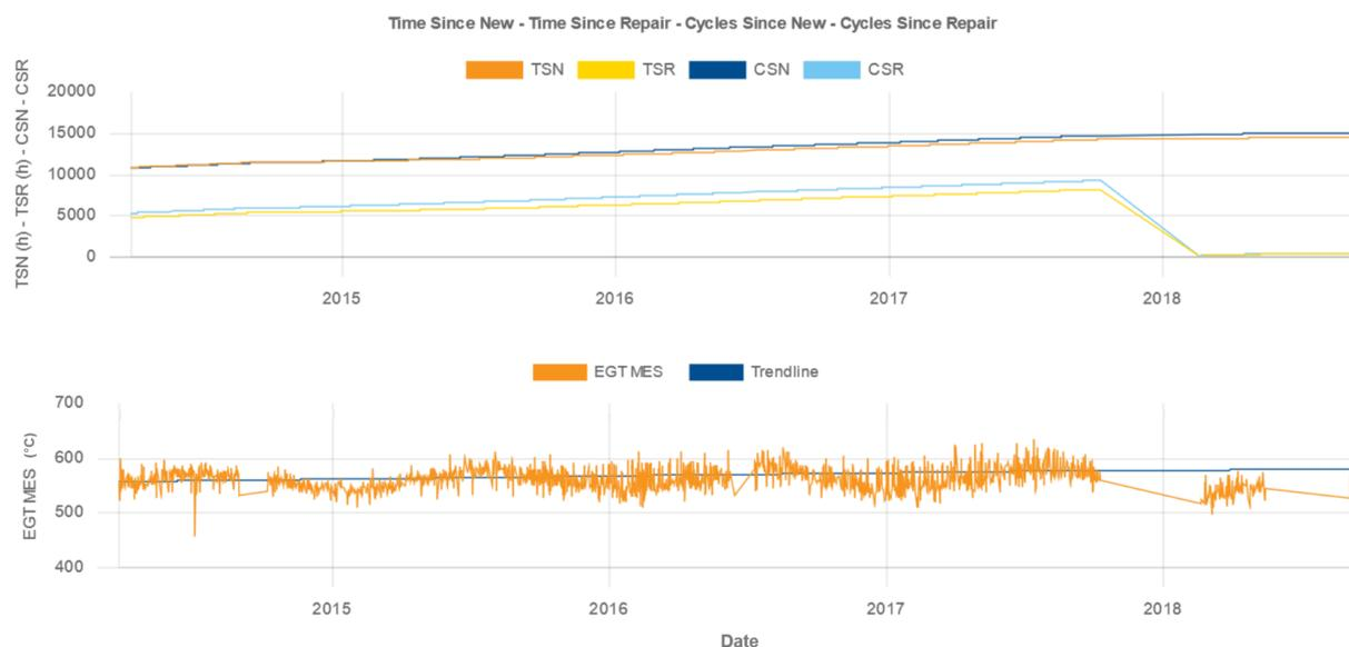
**Figure 1.6:** Typical performance tracking of an APU on the *Prognos for APU* system. The upper graph tracks the time and number of cycles since both the previous repair and the first cycle (new) of the APU while the lower chart tracks the EGT of the machine.
