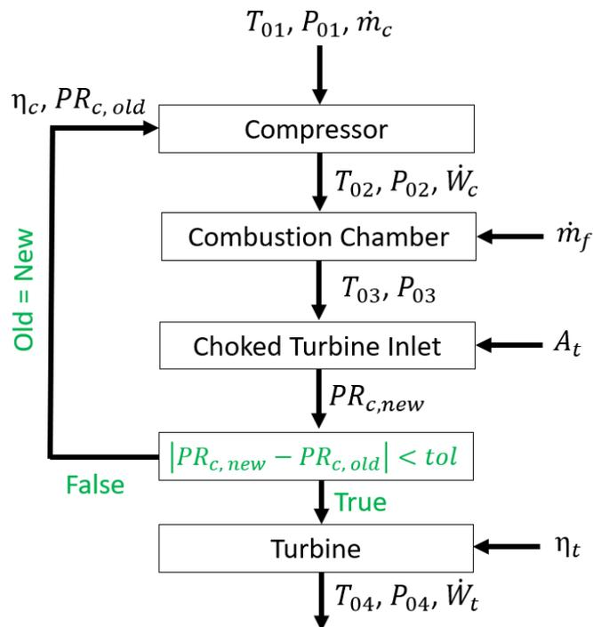
**Figure 4.5:** Calculation process for the on-design operation of a single-shaft gas turbine with a choked turbine inlet.
