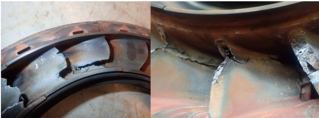
**Figure 8.12:** Deterioration in the first stage NGV of APU 1465 after removal due to high time
