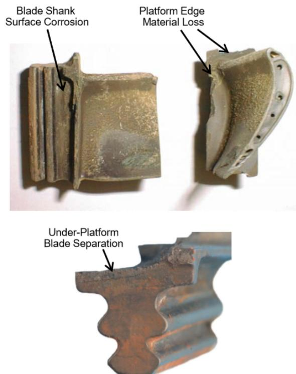
**Figure 2.3:** First stage turbine blades after extensive under-platform corrosion and crack growth [6].
