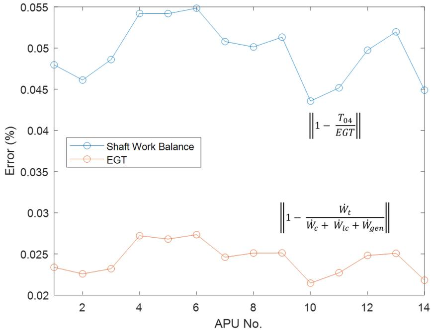
**Figure 5.8:** Residual error between both the measured and calculated EGT as well as that of the net-zero shaft power balance for the fourteen Honeywell 331-500 test runs at MES power condition.
