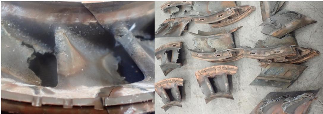
**Figure 8.6:** Deterioration in the first stage NGV after T1 blade failure for APUs 1608 (left) and 1308 (right).
