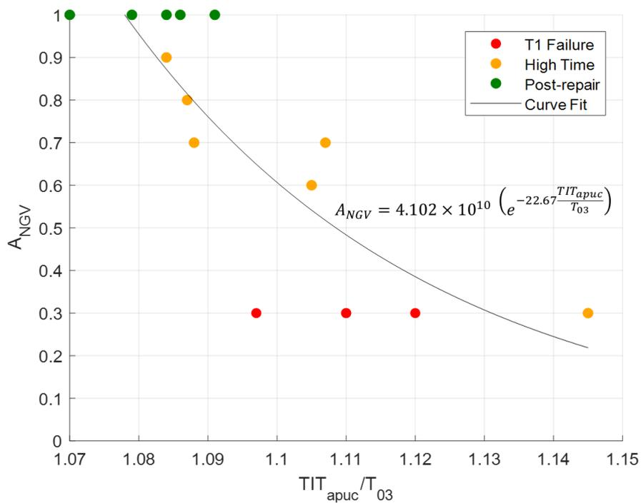
**Figure 8.21:** Relationship between the area of the first stage NGV and the ratio of controller- to model-calculated TIT for the Honeywell 331-500.
