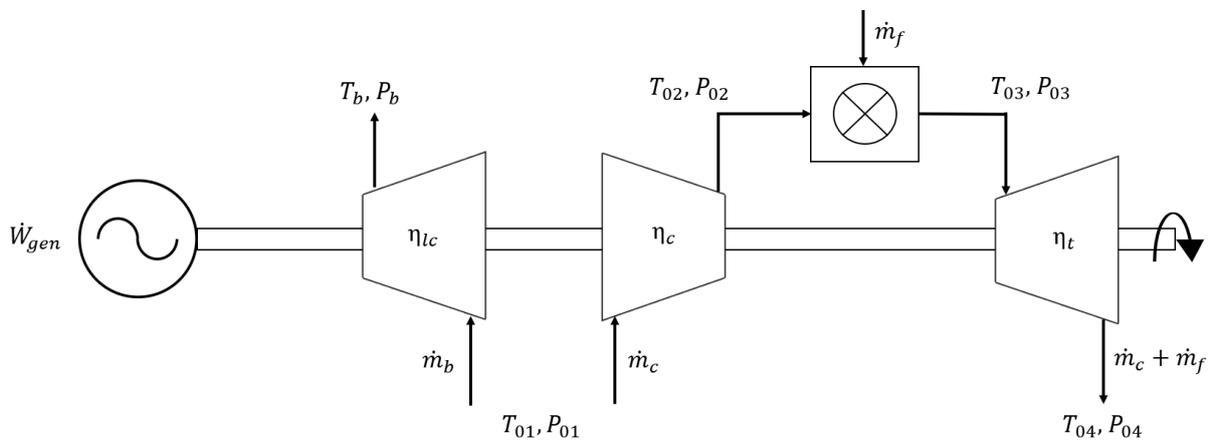
Figure 5.3: Schematic of the Honeywell 331-500 APU.
