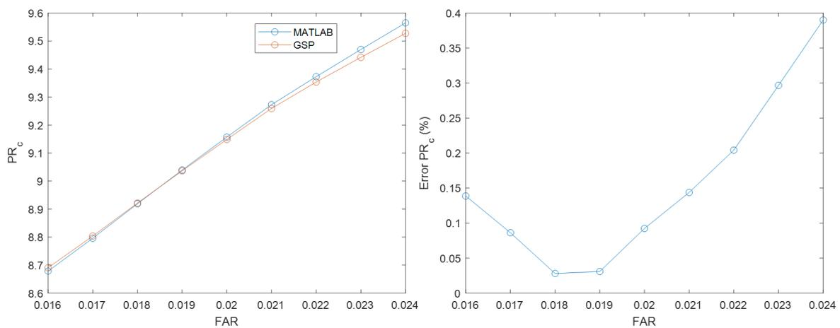
**Figure 4.8:** Comparison in compressor PR between the MATLAB and GSP models.
