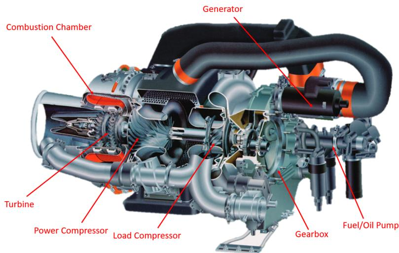
**Figure 1.2:** Cutaway diagram of a typical APU showing the main components of the machine [5].
