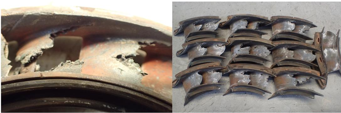
**Figure 8.5:** Deterioration in the first stage NGV after T1 blade failure for APUs 1602 (left) and 1552 (right).
