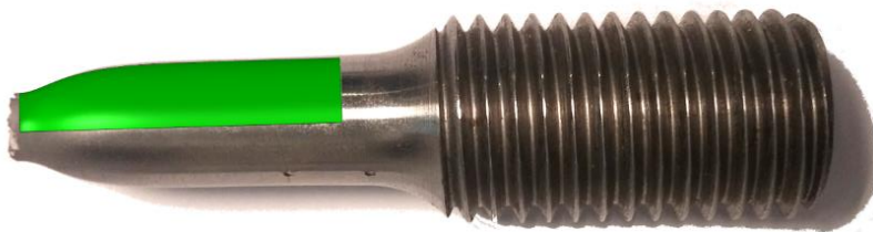
Figure 4-8 Deformed mesh overlaid on specimen.
