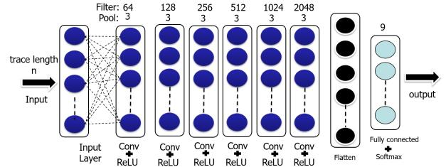
Fig. 1. Baseline CNN with its hyper-parameters
