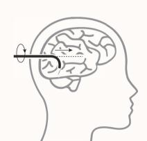
The principle of controlling a needle depends on a hypothesis which reads: "if the needle is pre-curved, the needle could be steered by translational and rotational movement towards a target."
