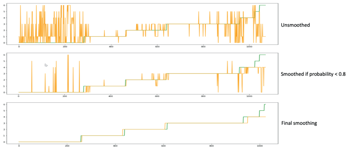
Figure 2.2: Example of smoothing of phases as created by COSMONiO, with the time-step on the x-axis and phase on the y-axis. The green line is the ground truth phase and the orange line is the predicted phase. This figure depicts a double smoothing, with the first N for the window set on 15 and the second on 11.
