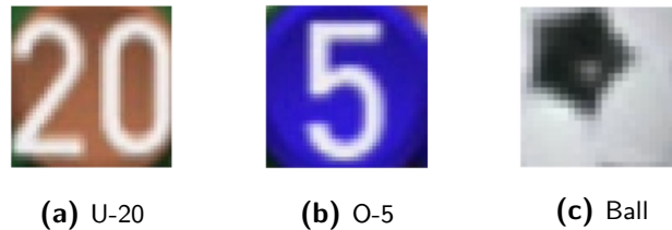
Figure 5-7: Examples of templates of players of opposing teams and the ball. Labels are given to each template, where the labels U-20 in (a) and O-5 in (b) refer to 'player #20 of the user team' and 'player #5 of the opposing team' respectively. The label in (c) refers to the ball.
