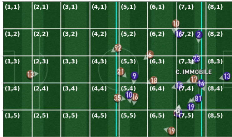
Figure 4-3: Field partitioning of the field into 40 regions of equal size. Each region is annotated with a specific discrete label, which is used for discretization purposes.
