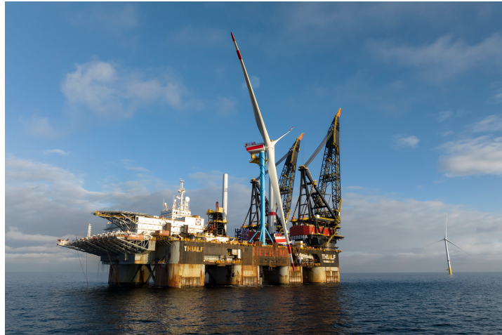
Figure 1.5: RNA fully assembled on the installation tower (in blue) on the Thialf's deck. Courtesy of Heerema Marine Contractors.
