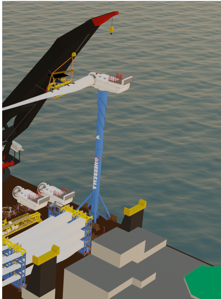
Figure 1.10: Representation of the GREP-less blade installation with a motion compensated Stewart platform connecting the blade / BIT to the crane's boom.
