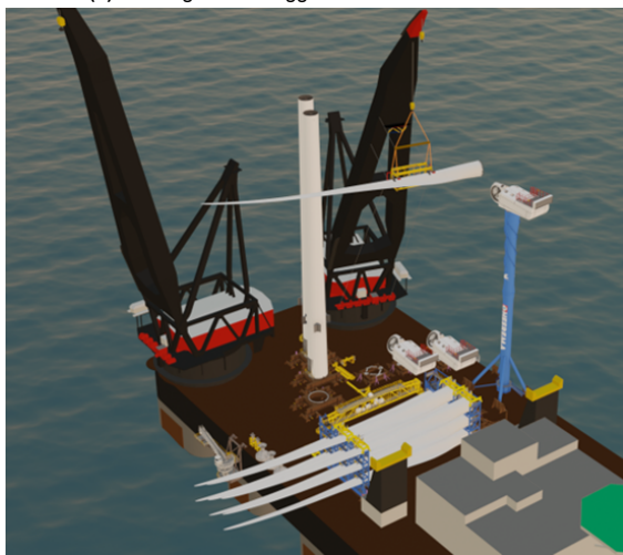
(c) Hoisting blade - tuggers #3 and #4 control BIT.
