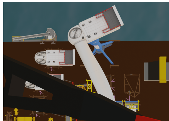
(b) Yawing the nacelle to free the blade from the BIT - top view.
