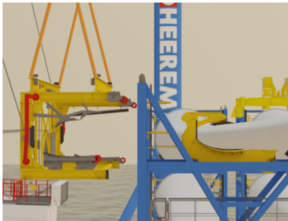
(a) BIT approach to blade - claws open.
