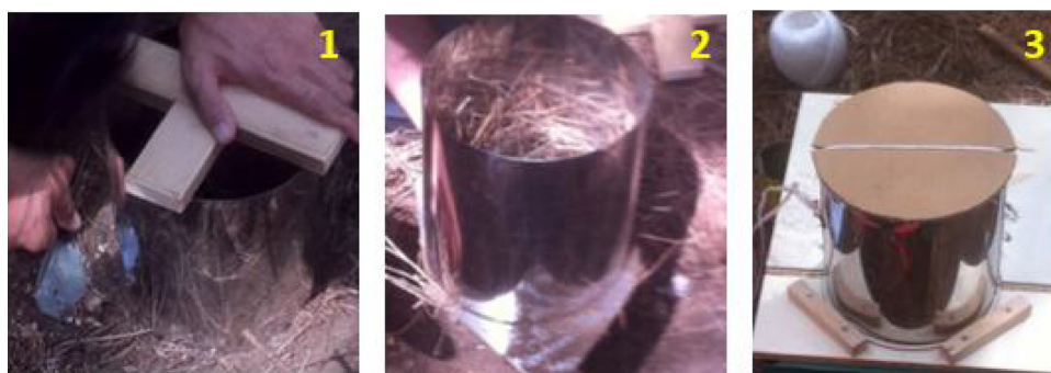
Fig. 2. Sampling phases (1–3) of litter and fermentation layer cores by an aluminium cylindrical collector designed to allow collecting “undisturbed” samples.
