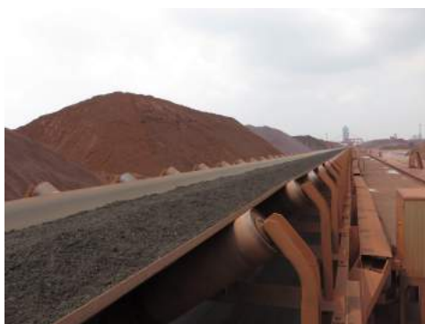
Figure 1.1: Part of a 1.5 km long belt conveyor system on a bulk terminal, figure courtesy of Rizhao Port Group Co., Ltd.
