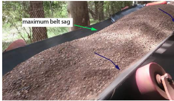
Figure 3.12: River sand within an idler spacing during conveyance.
