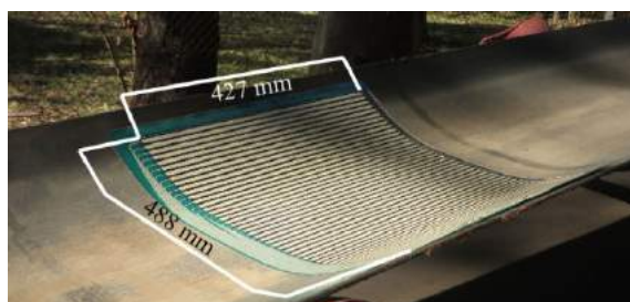
Figure 4.2: Tekscan pressure sensor model 5315.
