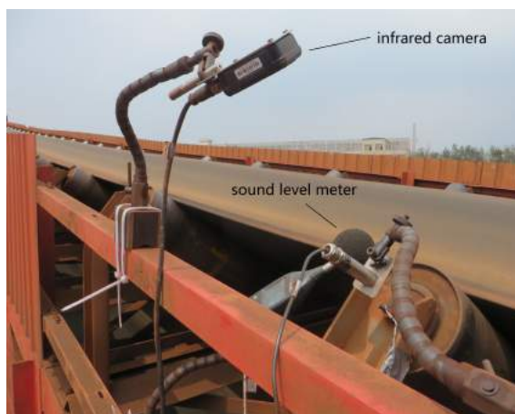
Figure 5.20: In-situ idler experimental setup.
