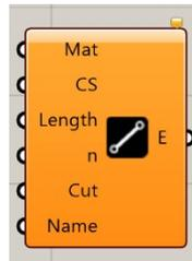
Figure 12 – Phoenix3D components defining the stock (Warmuth et al., 2021)
