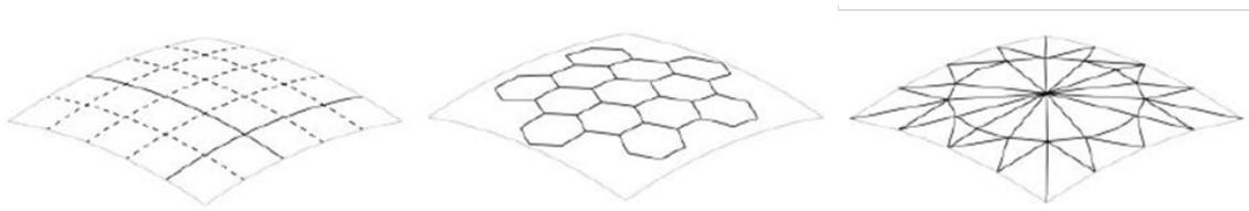
Figure 3 - diagrid, lattice and geodesic setup (Bouleau et al., 2019)
