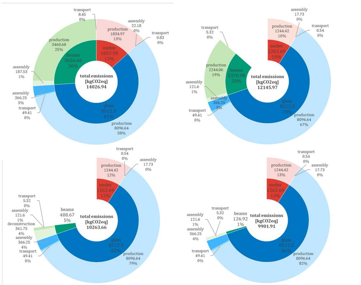
Figure 52 - top left: distribution of emissions for the single cross-section gridshell, top right: distribution of emissions for the cross-section optimized gridshell all new scenario, bottom left: distribution of emissions for the cross-section optimized gridshell all deconstruction scenario, bottom right: distribution of emissions for the cross-section optimized gridshell all stockpile scenario
