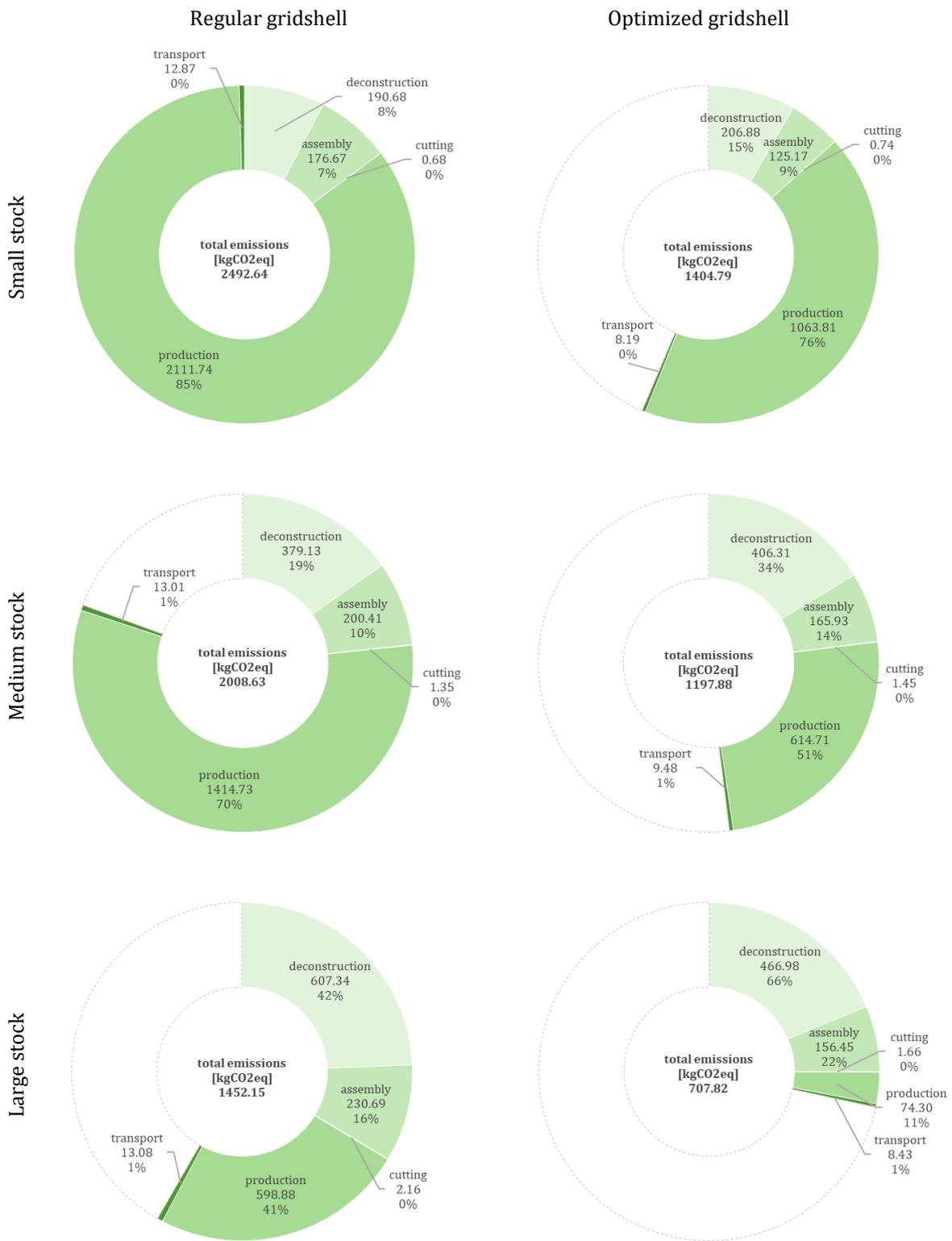
Figure 41 - distribution of the emissions for the beam members with different stock-sizes
